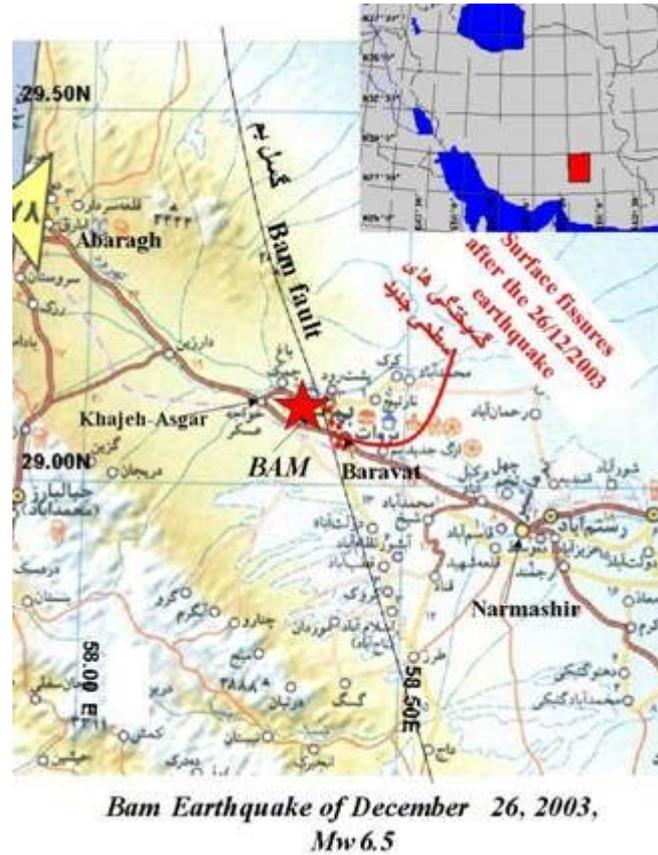
Figure-1: The location map of the epicenter and the reactivated Bam fault. The surface fissures created after Bam earthquake of 26/12/2003 are shown with dashed lines.
