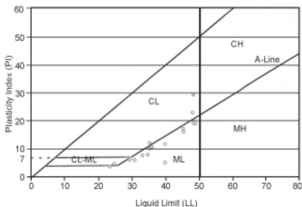
Figure 6. USCS classification of fine grained samples.
