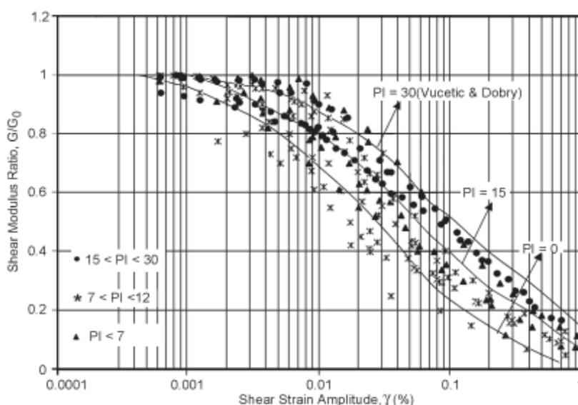
Figure 13. Shear modulus ratio of all tested materials.
