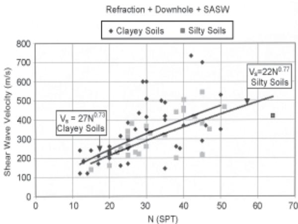
**Figure 3.** Correlation between  $V_s$  and N(SPT) for clayey and silty soils.
