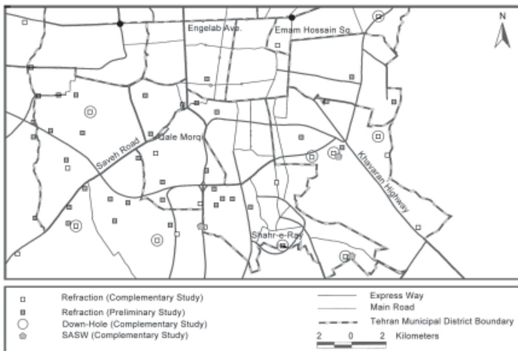
Figure 2. Location of geoseismic investigations.
