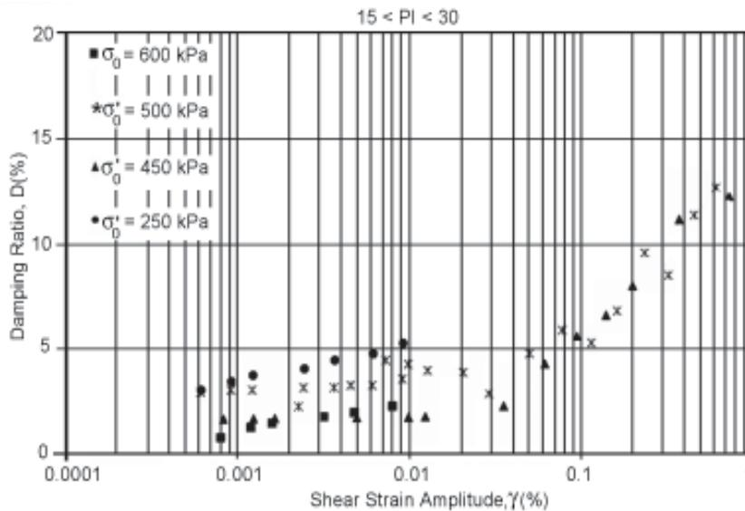
Figure 12. Damping ratio of medium plastic soils at different confining pressures.
