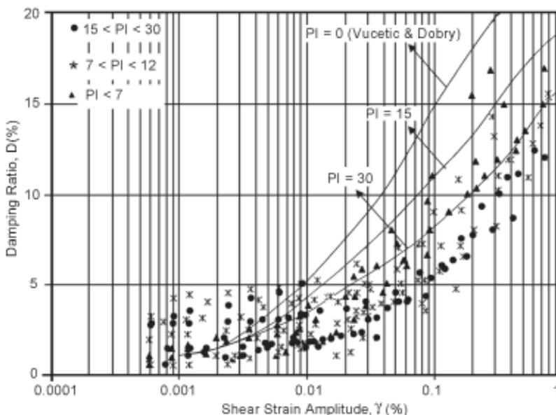
Figure 14. Damping ratio of all tested materials.
