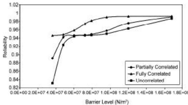
Figure 6. Effect of correlation of ground motion on the reliability (Soft soil).
