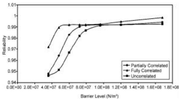
Figure 5. Effect of correlation of ground motion on the reliability (Firm soil).
