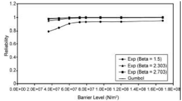
Figure 12. Effect of distribution of the magnitude of earthquake on the reliability (Soft soil).
