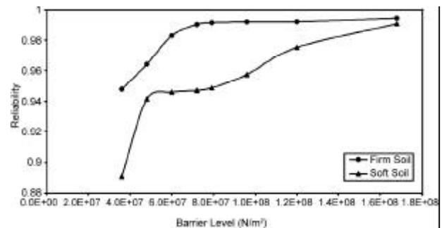
Figure 4. Effect of barrier level on the reliability.
