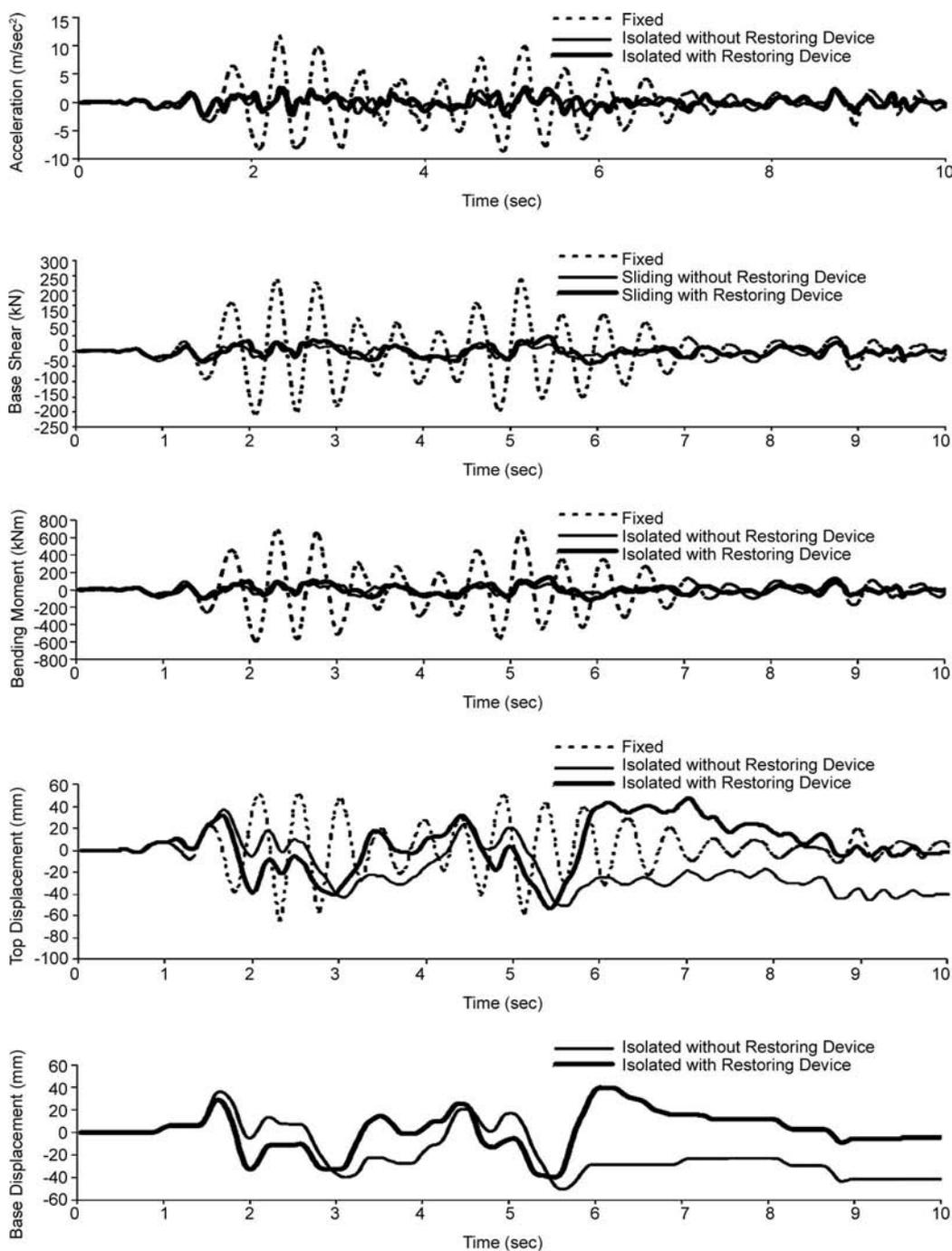
**Figure 2.** Variation of response with time for a structure subjected to El Centro earthquake.
