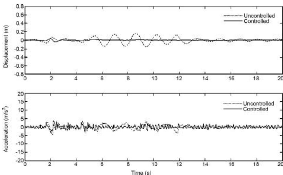
Figure 8. Flexible building responses to El Centro earthquake.
