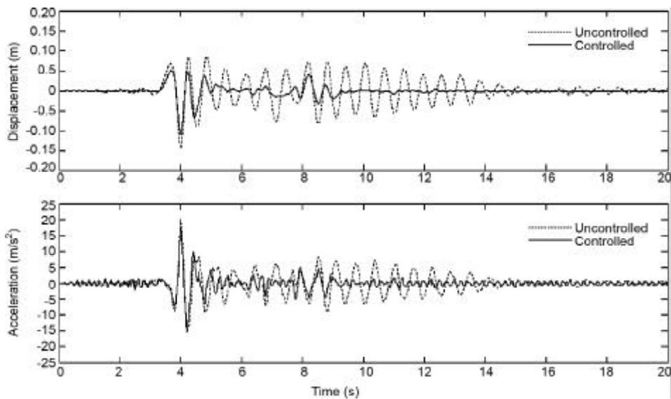
Figure 5. Rigid building responses to Northridge earthquake.
