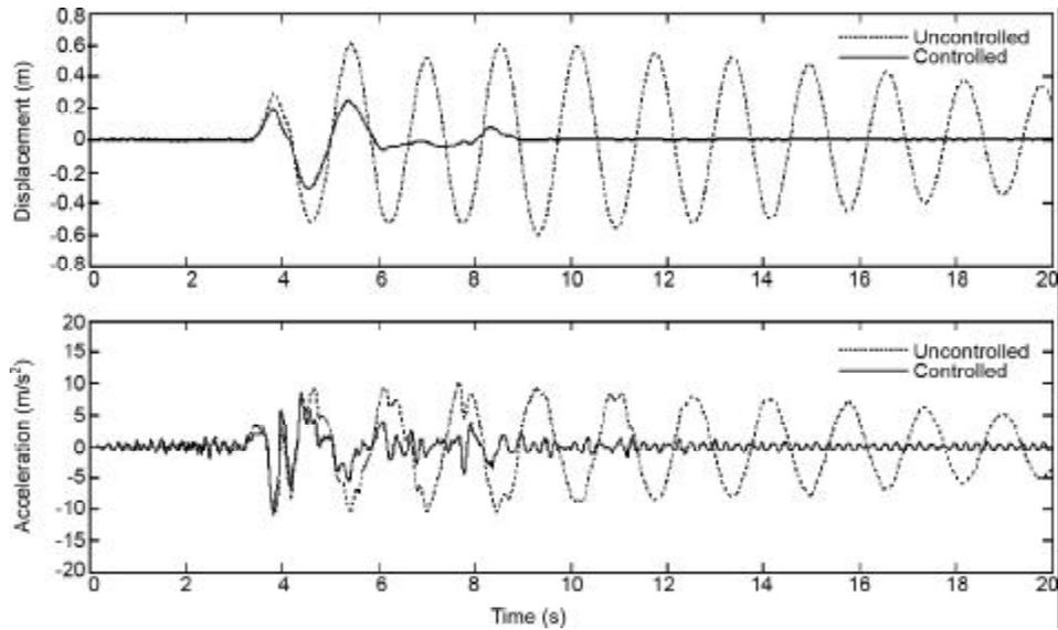
Figure 10. Flexible building responses to Northridge earthquake.
