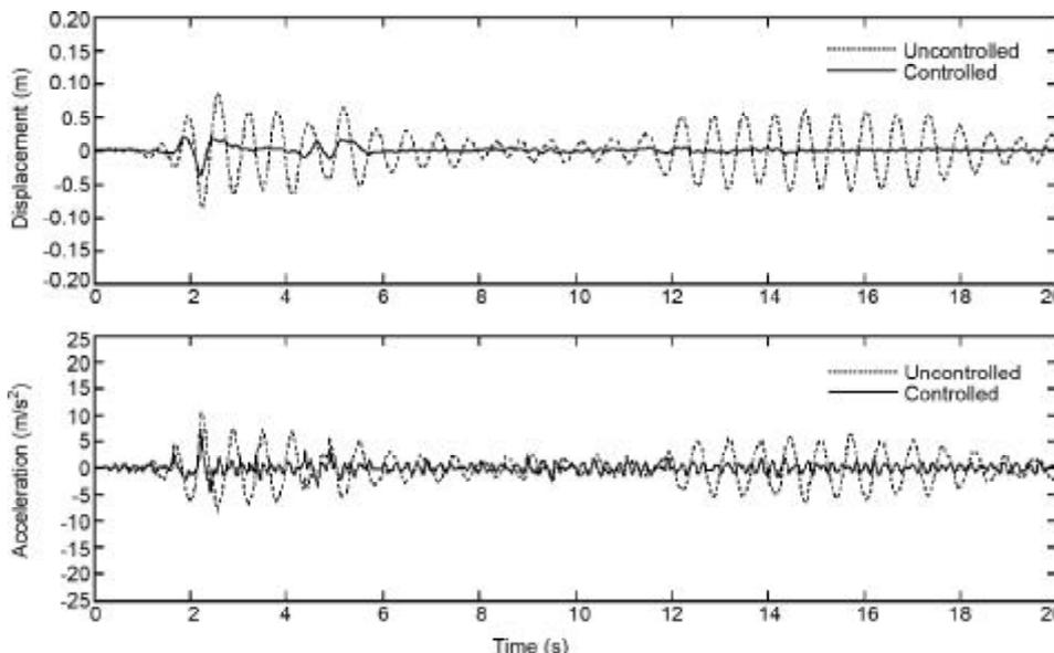
**Figure 3.** Rigid building responses to El Centro earthquake.
