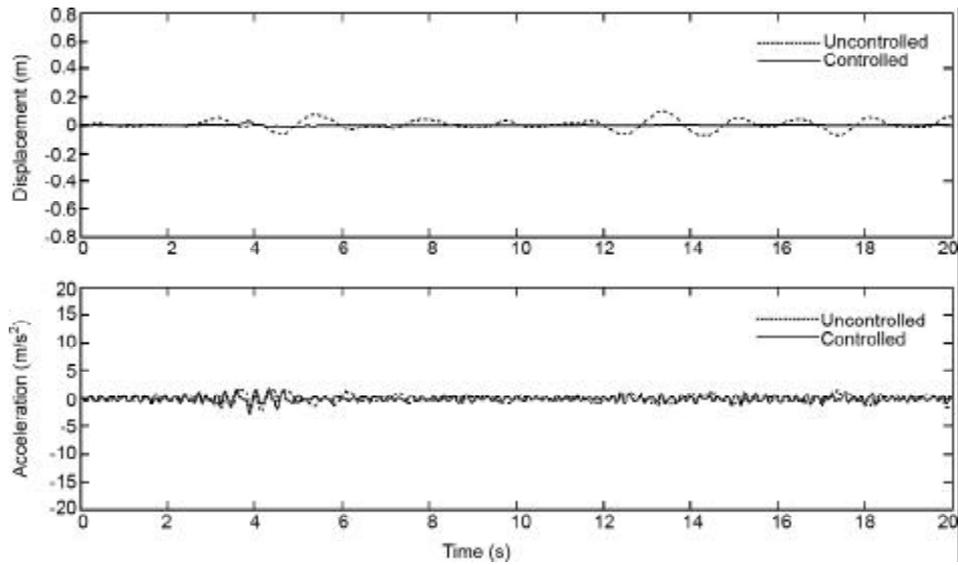
Figure 9. Flexible building responses to Hachinohe earthquake.
