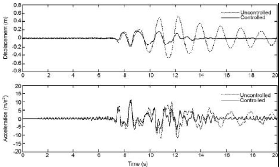
Figure 11. Flexible building responses to Kobe earthquake.
