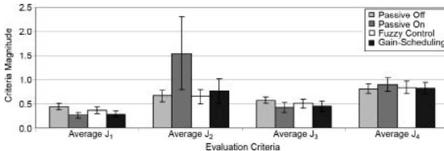
Figure 7. Comparison of average evaluation criteria values for the rigid structure's responses obtained with different control strategies (Error bars indicate 95% intervals).
