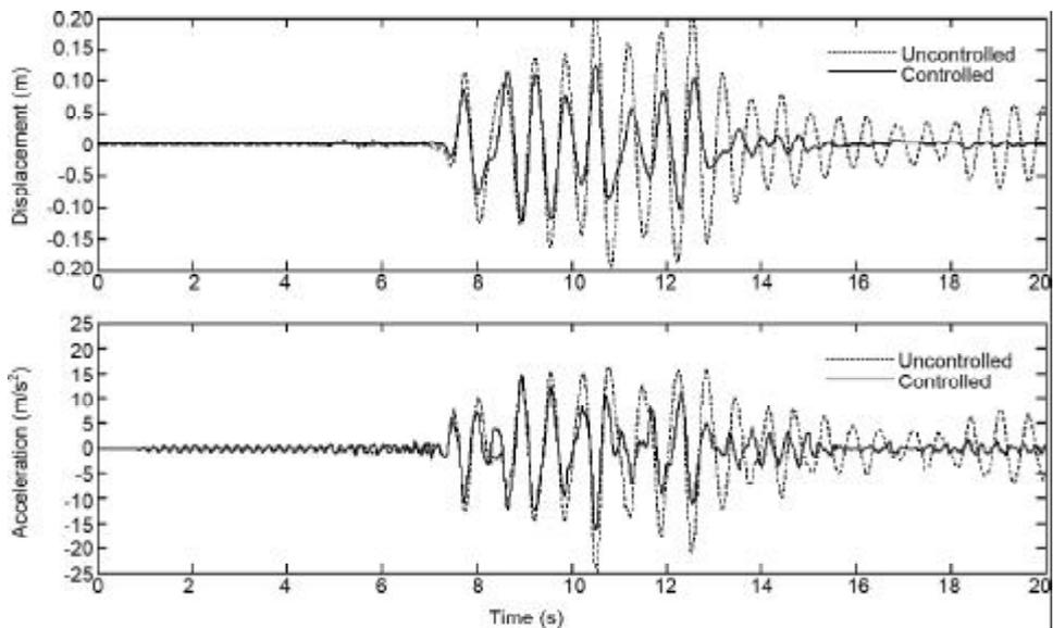
Figure 6. Rigid building responses to Kobe earthquake.
