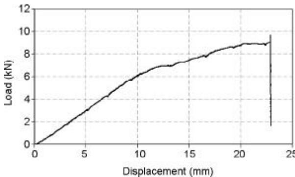
Figure 8. Out of plane load-displacement behavior of EIF-0.5.
