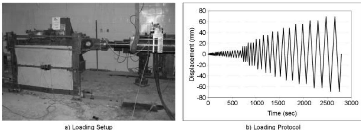
**Figure 3.** Loading setup and history of the specimens.
