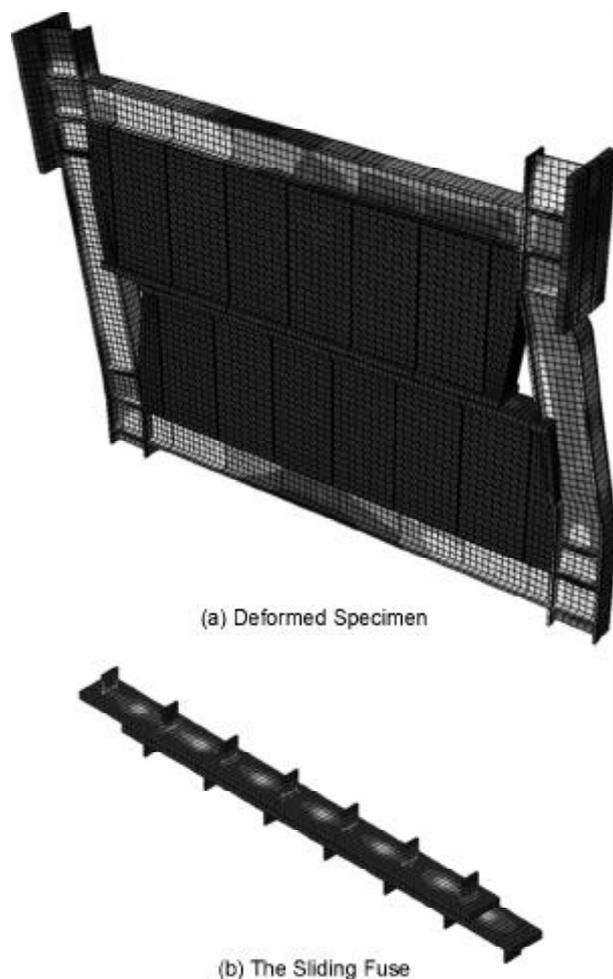
Figure 11. Deformation of the modelled specimen in ABAQUS.
