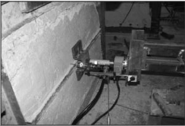
Figure 7. Out of plane loading test of EIF-0.5.
