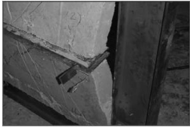
Figure 9. Out of plane deformation of EIF-0.5.
