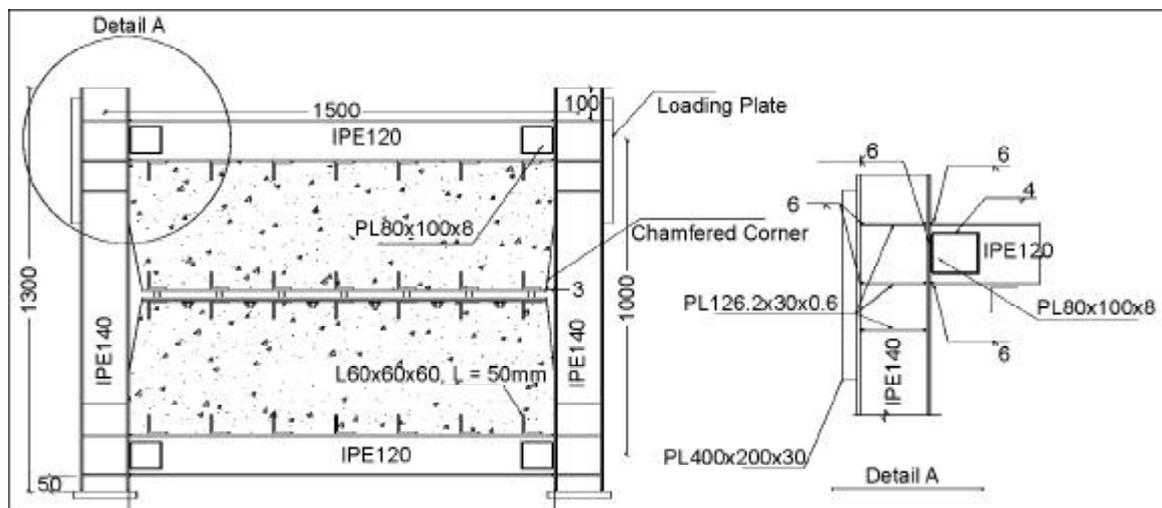
Figure 1. Details of the specimens' frame (dimensions in mm).
