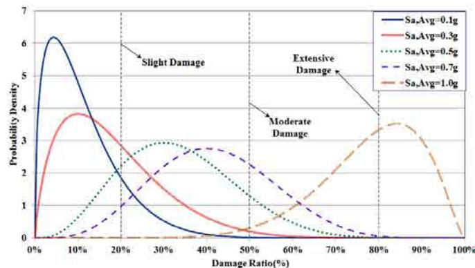
Figure 2. The probability density distribution of structural damage ratio with different intensities
