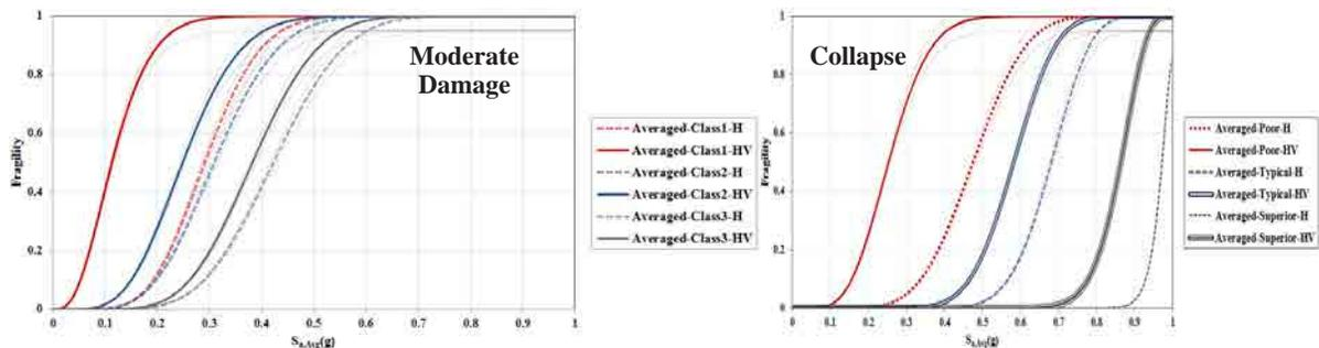
Figure 3. Averaged fragility curves for various subclasses in Moderate-damage and collapse modes
