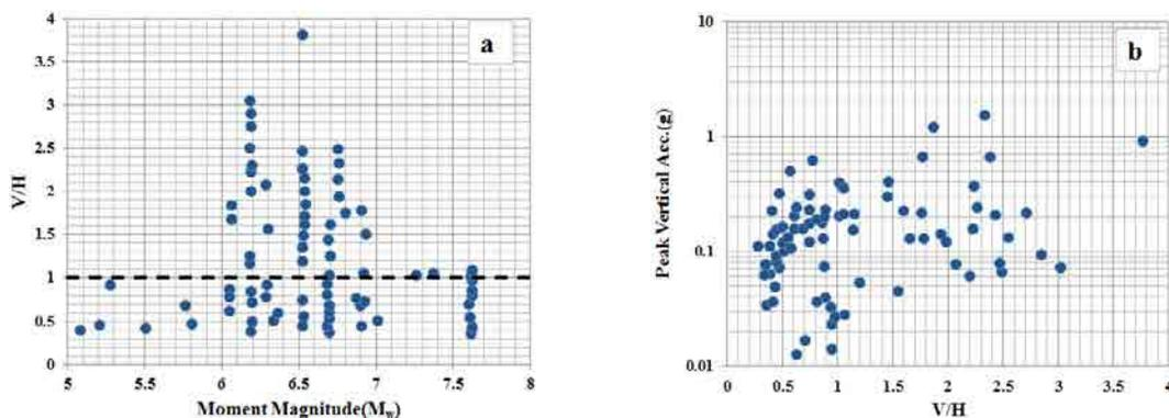
Figure 1. Ratios of peak vertical to horizontal acceleration (V/H) plotted against (a) moment magnitude, and (b) peak vertical acceleration (dashed line indicate the sample median)
