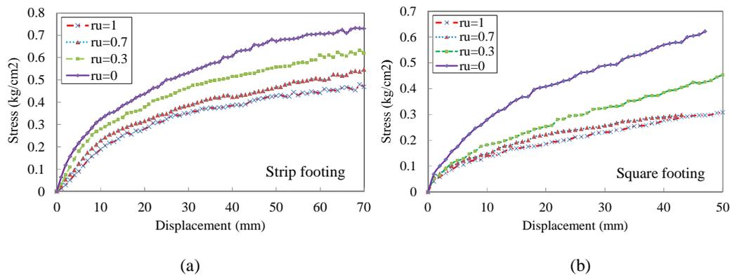
Figure 1. Stress-settlement curves in various levels of  $r_u$  for (a) strip foundation (b) square foundation
