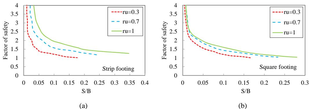
Figure 2. Curves of safety factor-normalized settlement for (a) strip foundation (b) square foundation
