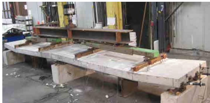
Figure 1. Final deflected shape of slab S1
