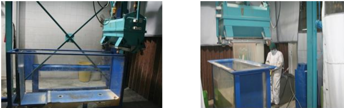
Figure 2. The 1-g model tests apparatus (left) and the pluviation technique with an electric sand rainer (right)
