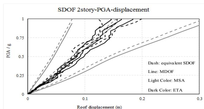
Figure 1. Response distribution of 2D MRF and its equivalent SDOF determined by MSA and ETA
