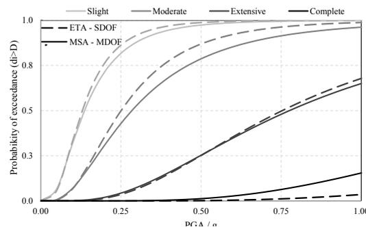
Figure 2. ETA and MSA obtained fragility curves for SDOF and MDOF respectively
