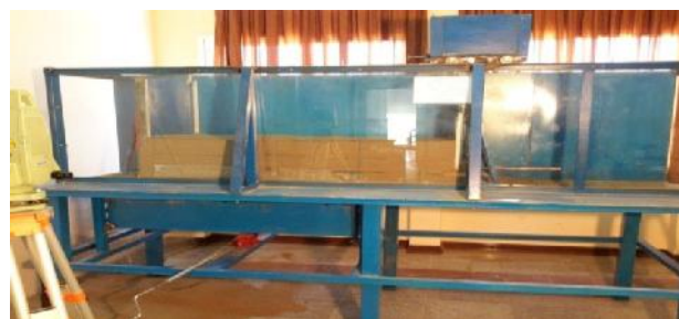
Figure 1. Overview of the reverse fault simulator
