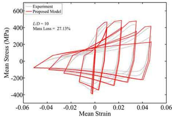
Figure 1. Comparison of the new phenomenological hysteretic model and experimental data
