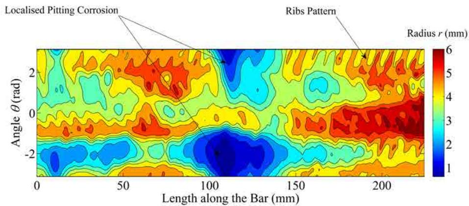
Figure 2. Corrosion pattern of a corroded bar with 54.23% mass loss
