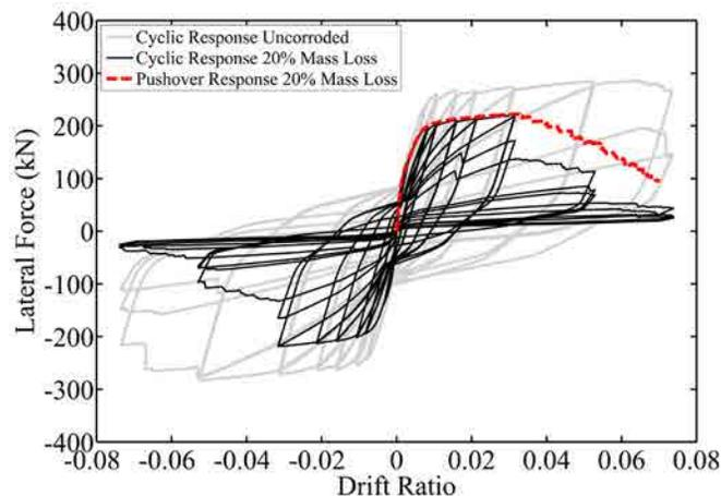
Figure 3. An example of the predicted response of a corroded column with 20% mass loss
