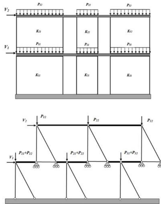
Figure 7. Equivalent truss model for combination of piers in elevation
