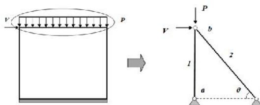
Figure 2. Equivalent truss model for an URM wall
