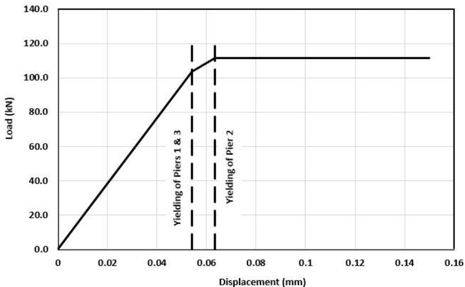
Figure 6. Push over curve of the wall obtained with equivalent truss method
