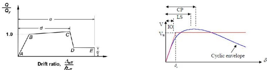
Figure 1. a- Standard plastic hinge for URM piers in FEMA 356 b- Elastoplastic load displacement curve used by Akhavesissy (2012)
