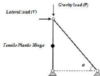
Figure 3. Definition of characteristic properties of equivalent truss model
