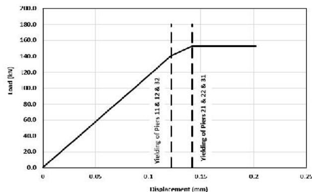
Figure 8. Push over curve of the 2 stories wall obtained with equivalent truss method
