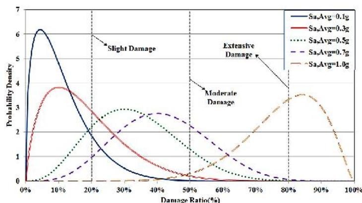
Figure 7. The probability density distribution of structural damage ratio with different intensities
