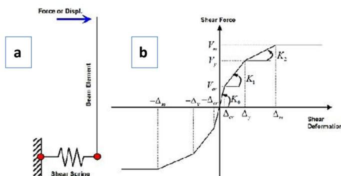
Figure 4. Shear spring modeling in Zeus-NL
