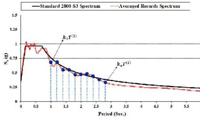
Figure 5. Schematic definition of  $S_{a,avg}$  based on the selected strong motion records
