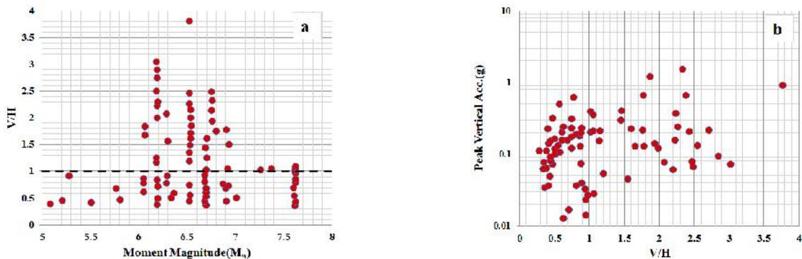
Figure 1. Ratios of peak vertical to horizontal acceleration (V/H) plotted against (a) moment magnitude, and (b) peak vertical acceleration (dashed line indicate the sample median)
