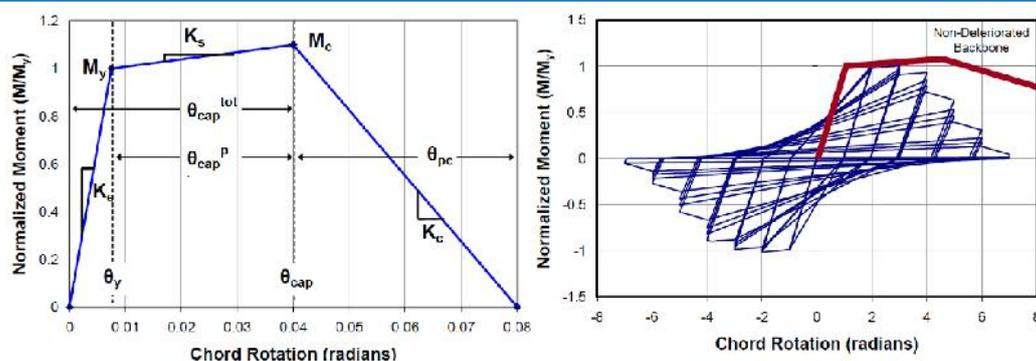
Figure 3. Monotonic and cyclic behavior of component model used in study. (Developed by Ibarra et al. (2005))
