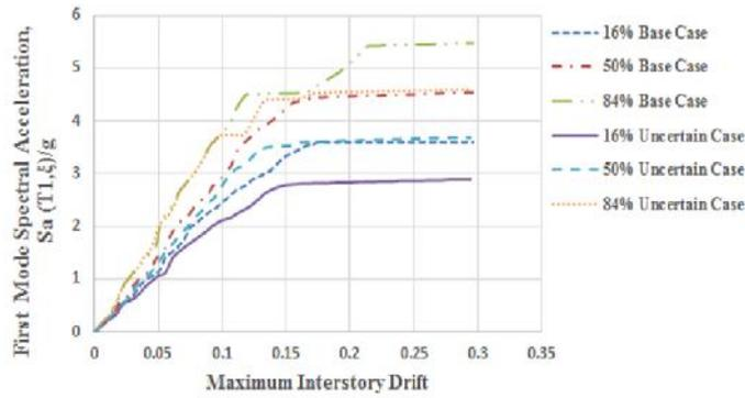
Figure 3. Summarized IDA curves for deterministic structural model (Base Case) and uncertain structural model (Uncertain Case)
