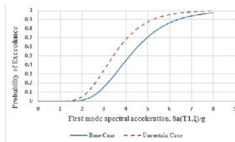
Figure 6. Fragility curves of Base and Uncertain cases for GI limit state
