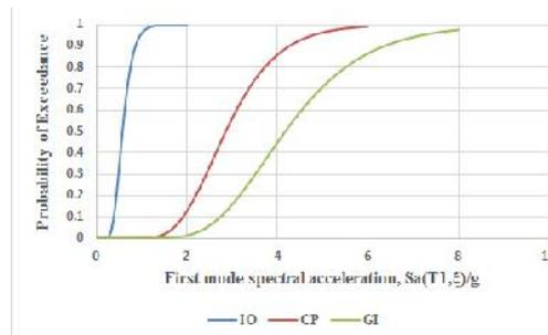
Figure 7. Fragility curves of different performance limit states in comparison
