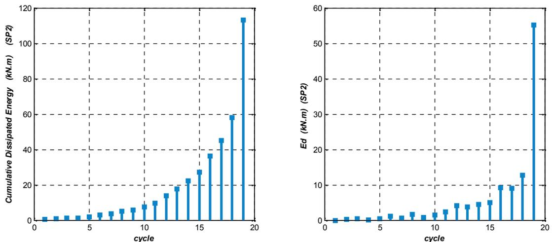
Fig 8. Dissipated energy in each cycle and cumulative dissipated energy of the SP2
