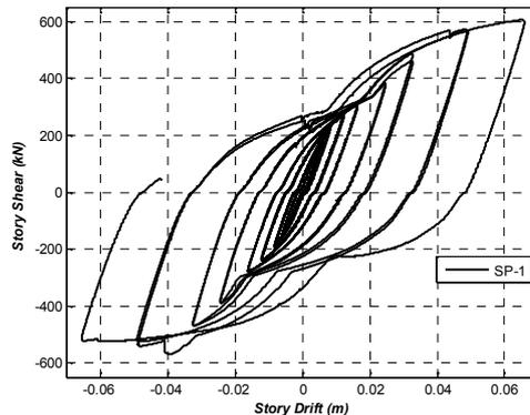
Fig. 4. Hysteretic response of specimen SP-1
