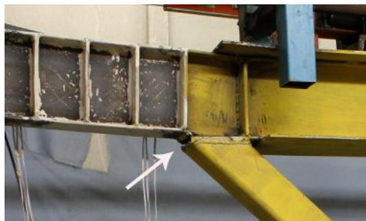
Fig. 6. Brace to link connection fracture during Cycle 19
