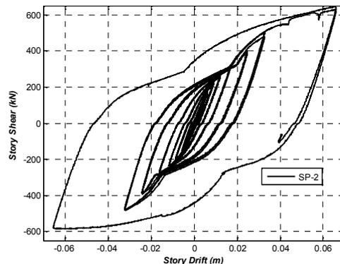
Fig. 5. Hysteretic response of specimen SP-2
