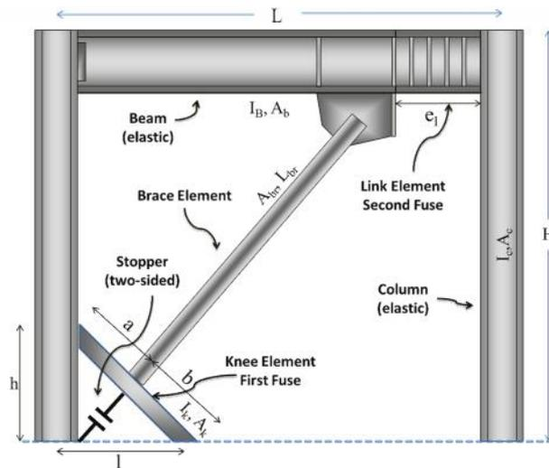
Figure 1. The proposed frame configuration.
