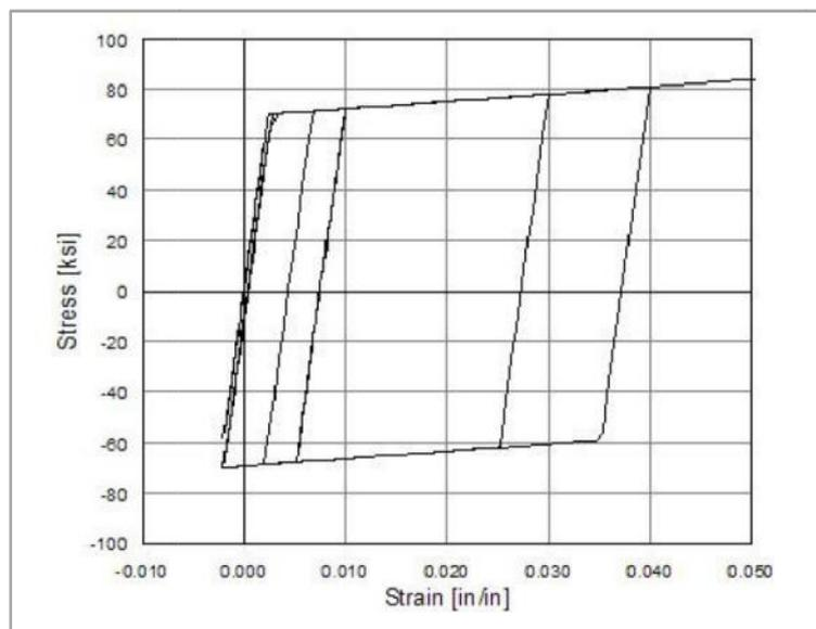
Figure 1. Hysteretic behavior of Steel01 material(Mazzoni et al., 2007)
