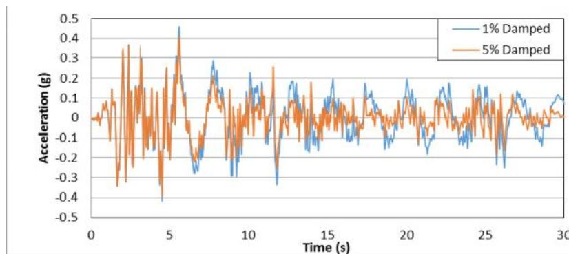
Figure 8. The acceleration at the top of the tower for the 1940 El Centro earthquake
