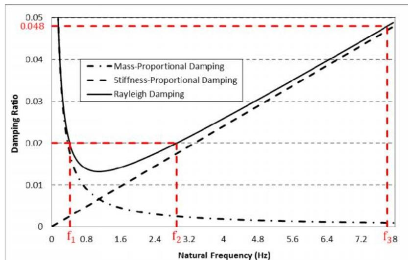
Figure 9. Modal damping ratios for calculation of Rayleigh damping matrix
