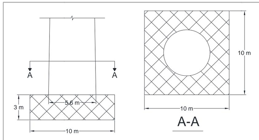
Figure 4. The dimensions related to the designed foundation for interaction models
