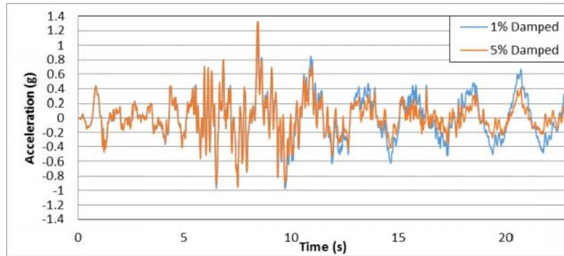
Figure 7. The acceleration at the top of the tower for the 1978 Tabas earthquake
