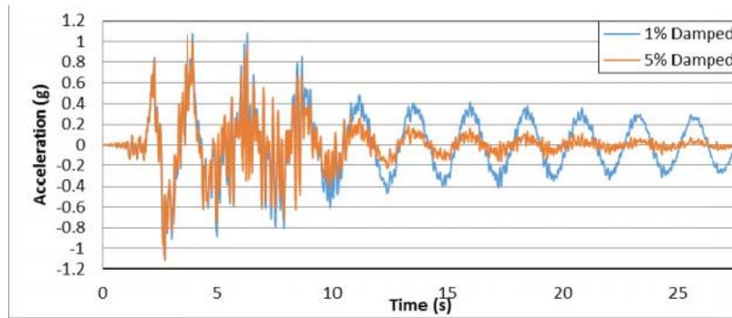
Figure 6. The acceleration at the top of the tower for the 2003 Bam earthquake
