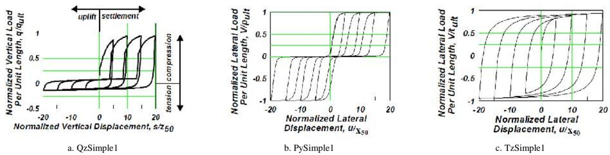
Figure 3. The backbone curves of soil models (Boulanger, 2000)
