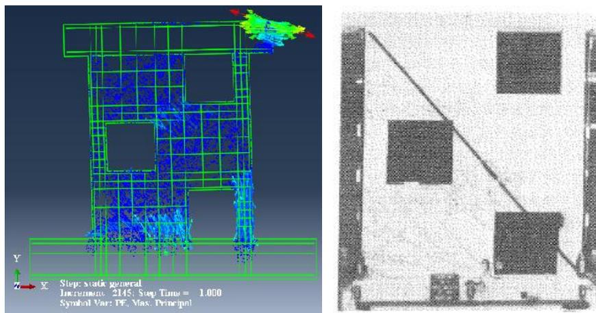
Figure 4. Cracking pattern of S2 specimen numerical model (left) and experimental wall of Yanez et al. (1991) (right)
