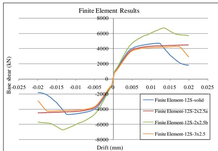
Figure 5. Load-drift curves of finite element results
