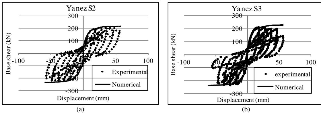
Figure 3. Comparison of load- displacement curve of experimental models of Yanez et al. (1991) and numerical results
