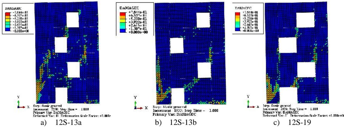
Figure 6. Contour plot of compression damage
