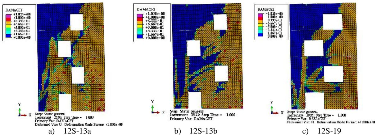
Figure 7. Contour plot of tension damage
