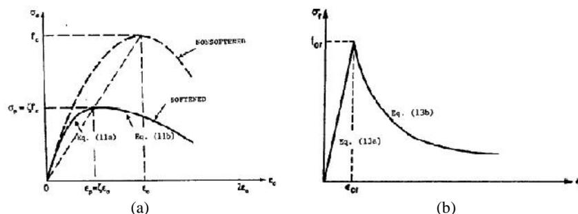
Figure 2. a) Compression stress-strain curve of concrete b) Tensile stress-strain curve of concrete (Belarbi et al., 1996)
