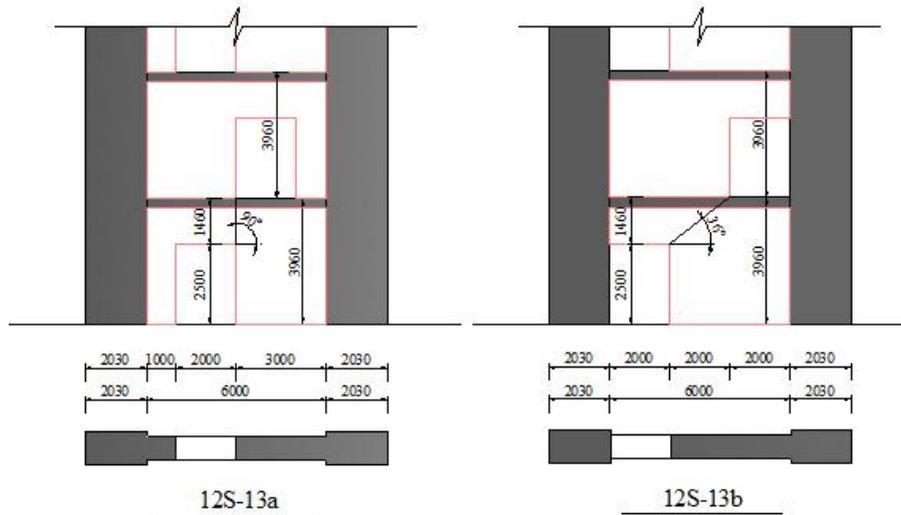
Figure 5. 12S-13a and 12S-13b wall scheme (Notations of dimensions in mm)
