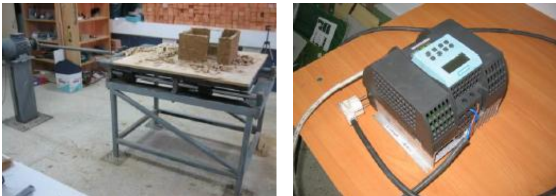
Figure 2. shaking table test setup and controller (Ersubasi and Korkmaz, 2010)
