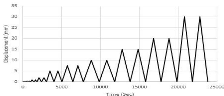
Figure 8. Loading protocol of the out-of-plane testing
