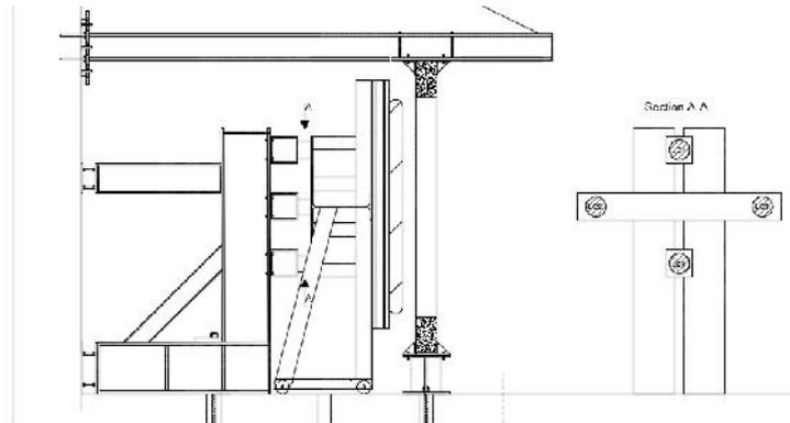
Figure 6. Configuration adopted for the loadcells
