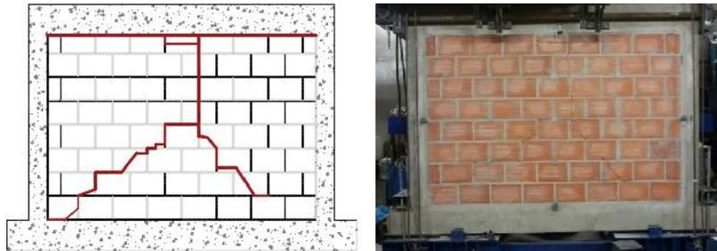
Figure 12. Crack pattern of the infilled frame
