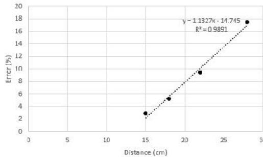
Figure 10. Decrease in effective area of airbag by increasing its distance from wooden board
