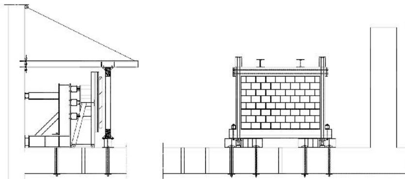
Figure 5. Test setup for out-of-plane testing
