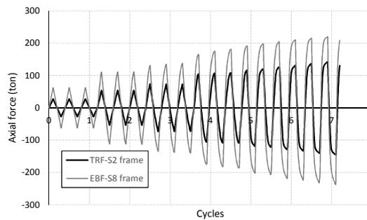
Figure 5. Side columns axial load responses of TRF and EBF frames along cyclic loading
