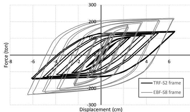
Figure 7. Hysteretic curve of one TRF and one EBF frame
