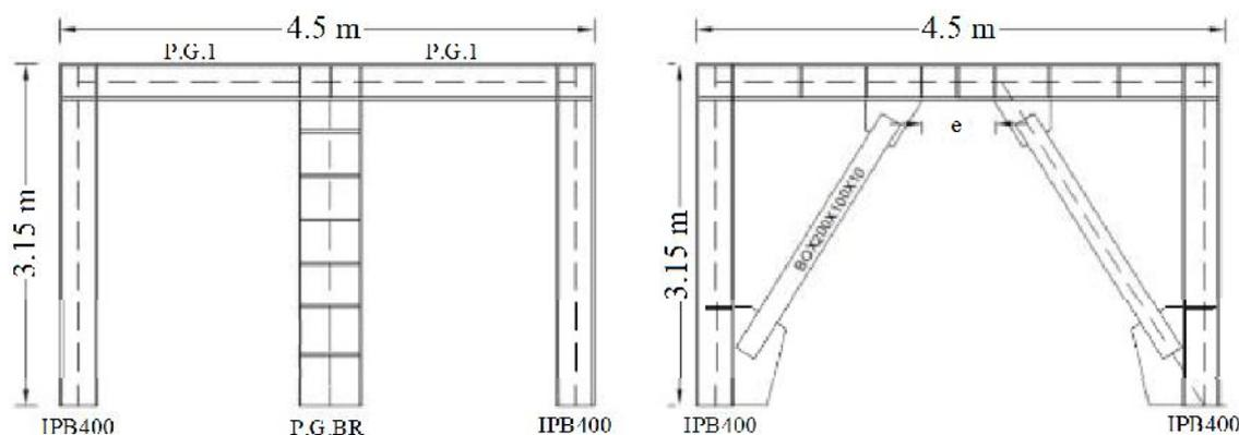
Figure 2. Typical T-shape resistant frame (at left) and eccentrically braced frame (at right)
