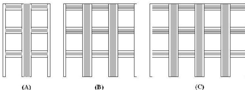
Figure 1. Types of TRF frames with one, two and three vertical members
