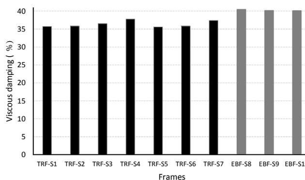
Figure 8. Viscous damping of TRF and EBF frames
