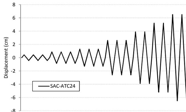
Figure 3. Cyclic loading protocol applied as displacement (SAC-ATC24)
