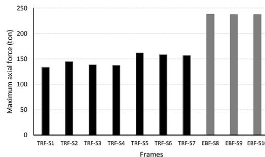
Figure 6. Maximum side columns axial load responses of all TRF and EBF frames
