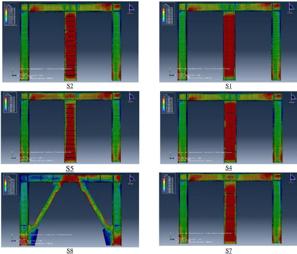
Figure 4. Vonmises stress distribution in the S1, S2, S4, S5, S7 and S8 frames
