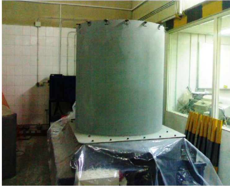
Figure 1. A view of the installation of tank model on the shaking table
