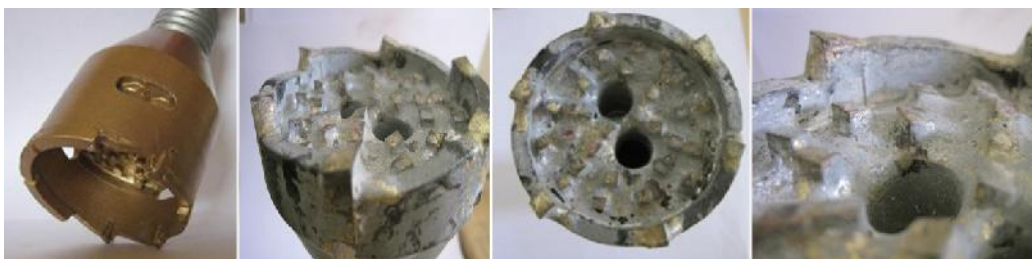
Figure 6. The combined coring & non-coring bit
