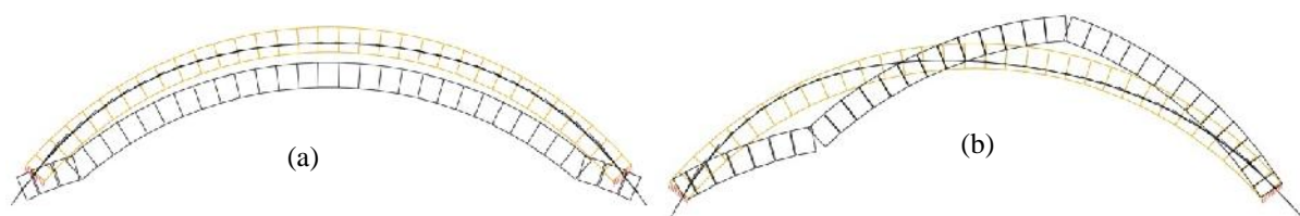
Figure 5. Failure mechanism and trust line of reference vault developed by Block2D software. a) Under gravity load. b) Under horizontal loading
