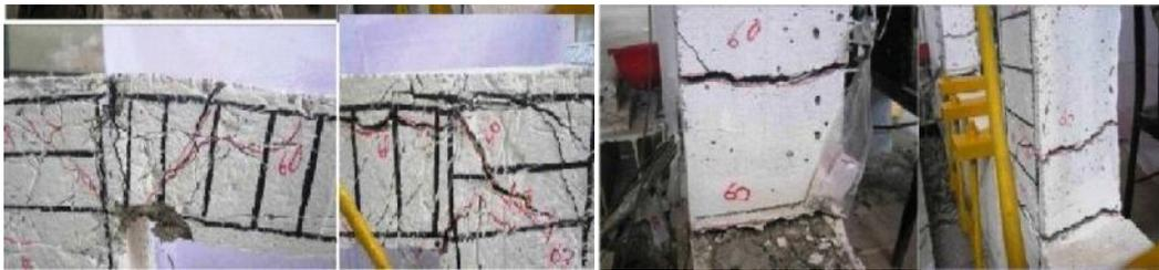
Figure 4. Location of cracks and tensile cracks pattern in experimental model by Hemati (2012)
