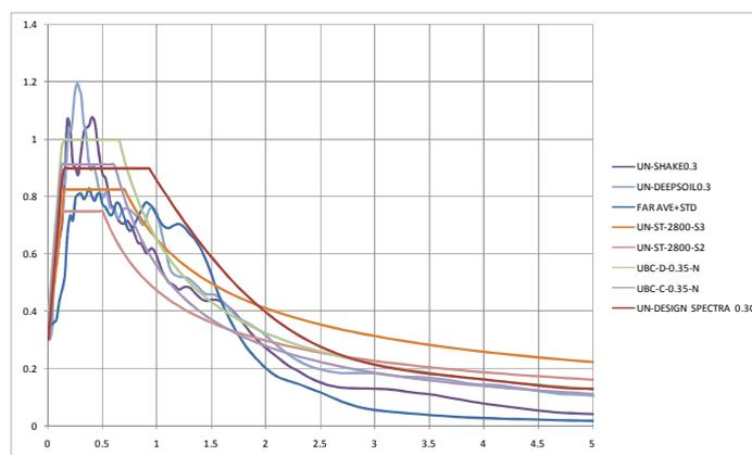
Figure 4. Proposed non-scaled site-specific design spectra for corresponding peak acceleration (0.3g) with presented curves in comparison with Iranian Seismic design code (Standard, 2800) and UBC97 (with consideration of near-field effects)
