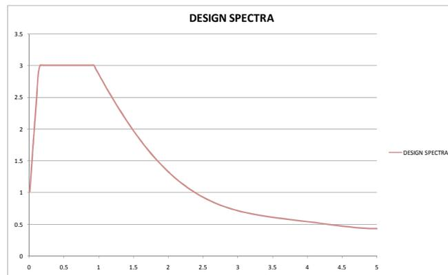
Figure 3. Proposed site design spectra
