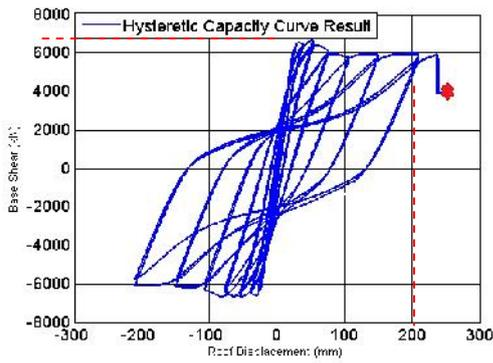
(a) Roof drift-base shear capacity curve
