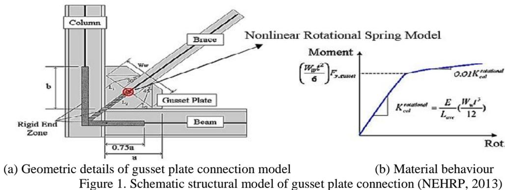
Figure 1. Schematic structural model of gusset plate connection (NEHRP, 2013)
