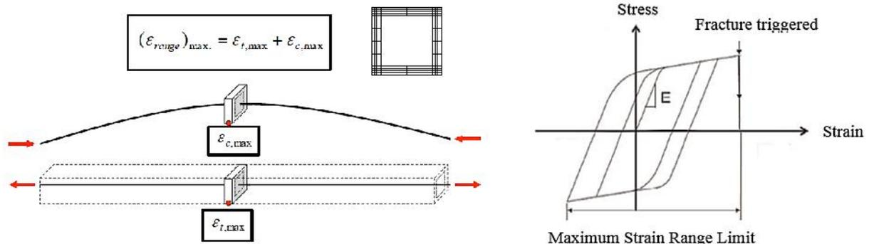
(a) Schematic of the midspan fiber section for brace model      (b) Schematic of the fracture material model
