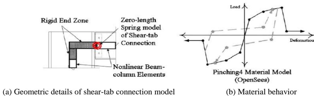
Figure 2. Schematic structural model of shear-tab connection (NEHRP, 2013)
