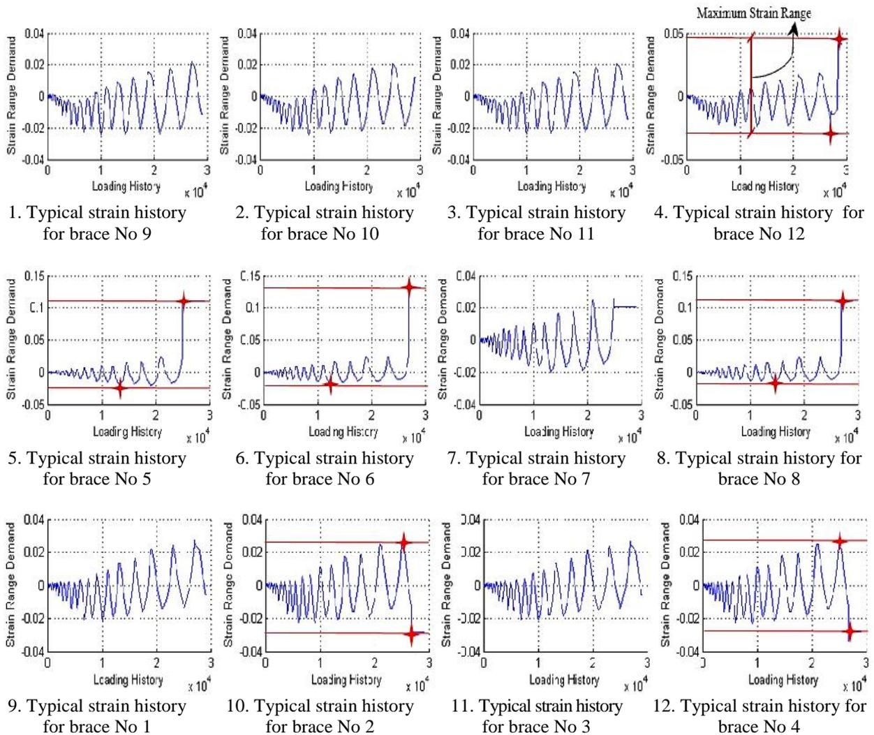
Figure 9. cumulative strain changes at the extreme fiber on the compression side of the hinge in the middle
