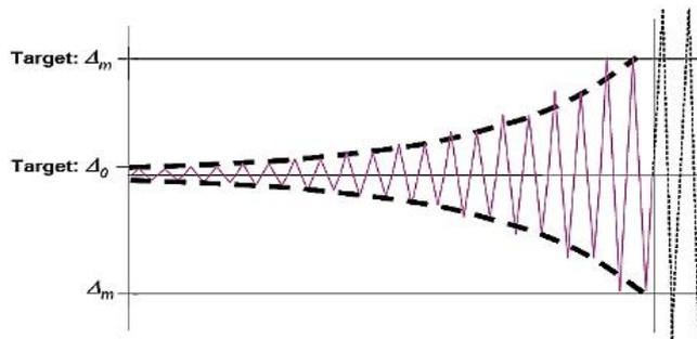
Figure 7. Sketch of displacement-controlled loading history [19]
