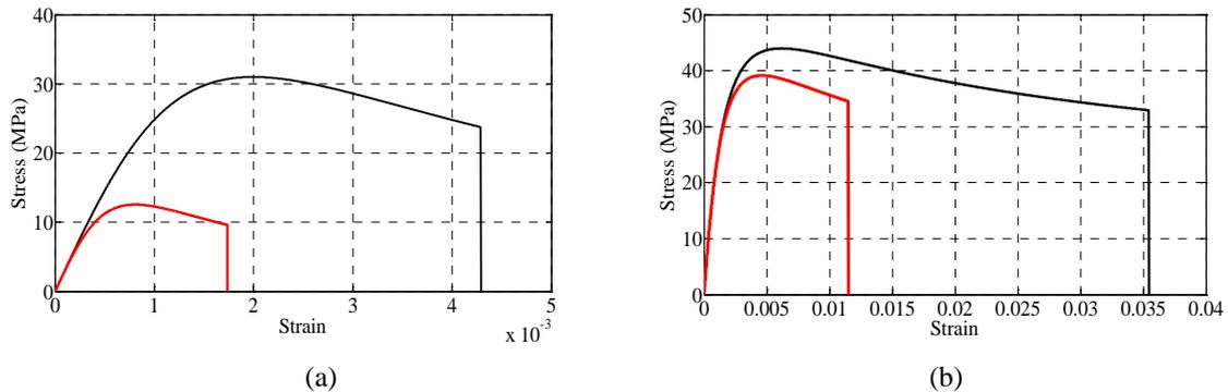
Figure 4. Material model of concrete: (a) unconfined cover concrete (b) confined core concrete
