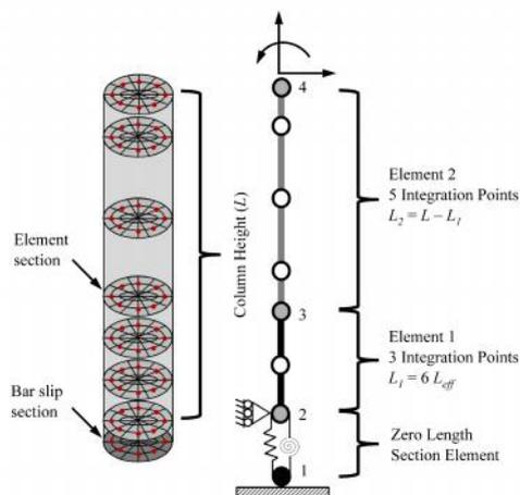
Figure 1. Proposed nonlinear fibre beam-column finite element model
