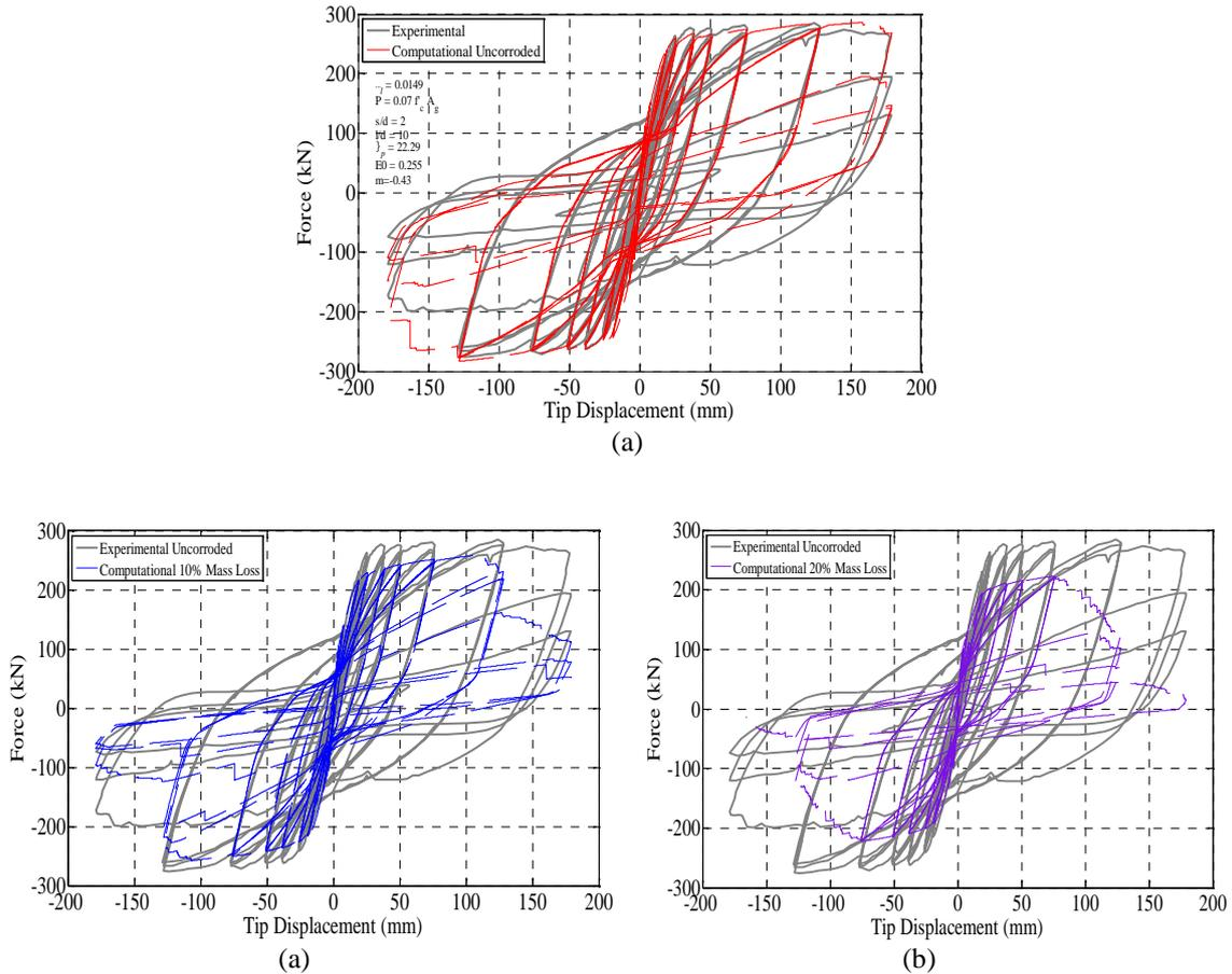
Figure 5. Nonlinear cyclic response of Lehman's column 415: (a) uncorroded (b) 10% mass loss and (c) 20% mass loss
