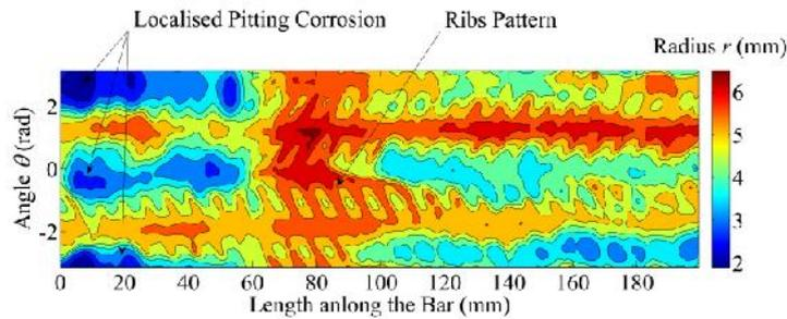
Figure 2. Contour plot of corrosion pattenr of a corroded bar with 36.40% mass loss
