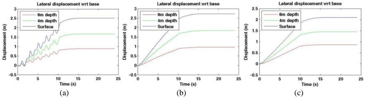
Figure 5. Lateral displacement: (a) 10 cycle, (b) 20 cycle, (c) 40 cycle, ( $k = 5e-4 \text{ m/s}$ , acceleration amplitude = 3)
