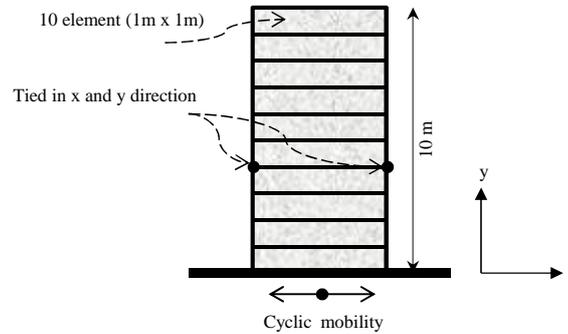
Figure 1. Soil column consists of 10 elements and relevant boundary conditions
