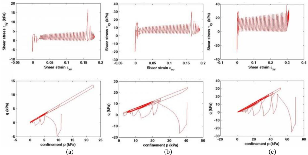
Figure 12. Shear stress  $\tau_{xy}$  VS. shear strain  $\epsilon_{xy}$  and confinement  $p$  VS. deviatoric stress  $q$  for (a) 2m depth, (b) 6m depth, (c) 10m depth, ( $k = 5 \times 10^{-6} \text{ m/s}$ , acceleration amplitude = 3, and 40 cycle)
