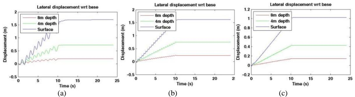
Figure 4. Lateral displacement: (a) 10 cycle, (b) 20 cycle, (c) 40 cycle, ( $k = 5e-3$  m/s, acceleration amplitude = 3)
