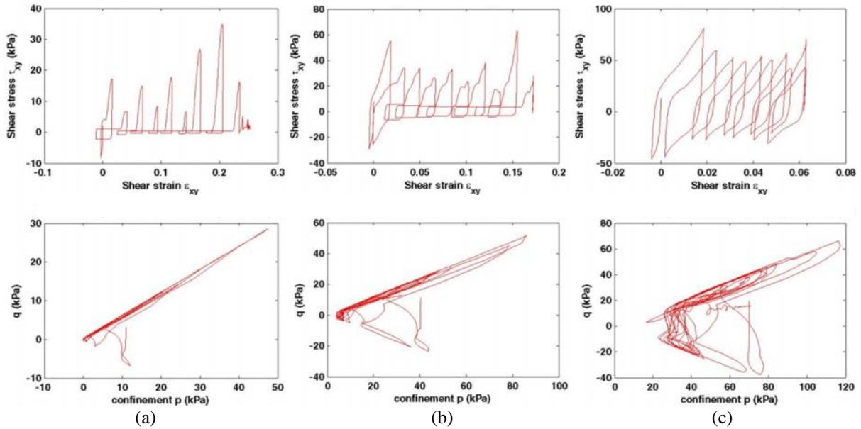
Figure 11. Shear stress  $\tau_{xy}$  VS. shear strain  $\epsilon_{xy}$  and confinement  $p$  VS. deviatoric stress  $q$  for (a) 2m depth, (b) 6m depth, (c) 10m depth, ( $k = 5 \times 10^{-3} \text{ m/s}$ , acceleration amplitude = 3, and 10 cycle)
