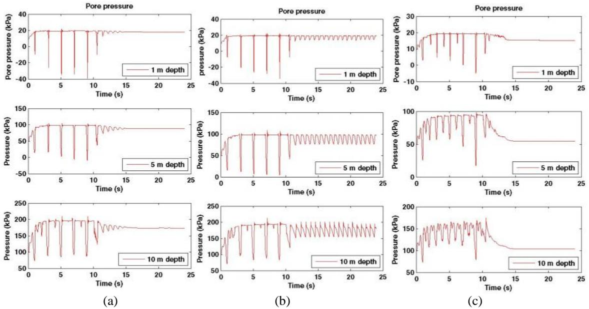
Figure 8. Excess pore pressure dissipation for (a)  $k = 5e-6 \text{ m/s}$ , (b)  $k = 5e-4 \text{ m/s}$ , (c)  $k = 5e-3 \text{ m/s}$ , (10 cycle, acceleration amplitude = 3)
