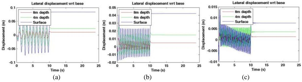
Figure 6. Lateral displacement: (a) 10 cycle, (b) 20 cycle, (c) 40 cycle, ( $k = 5e-3 \text{ m/s}$ , acceleration amplitude = 2)
