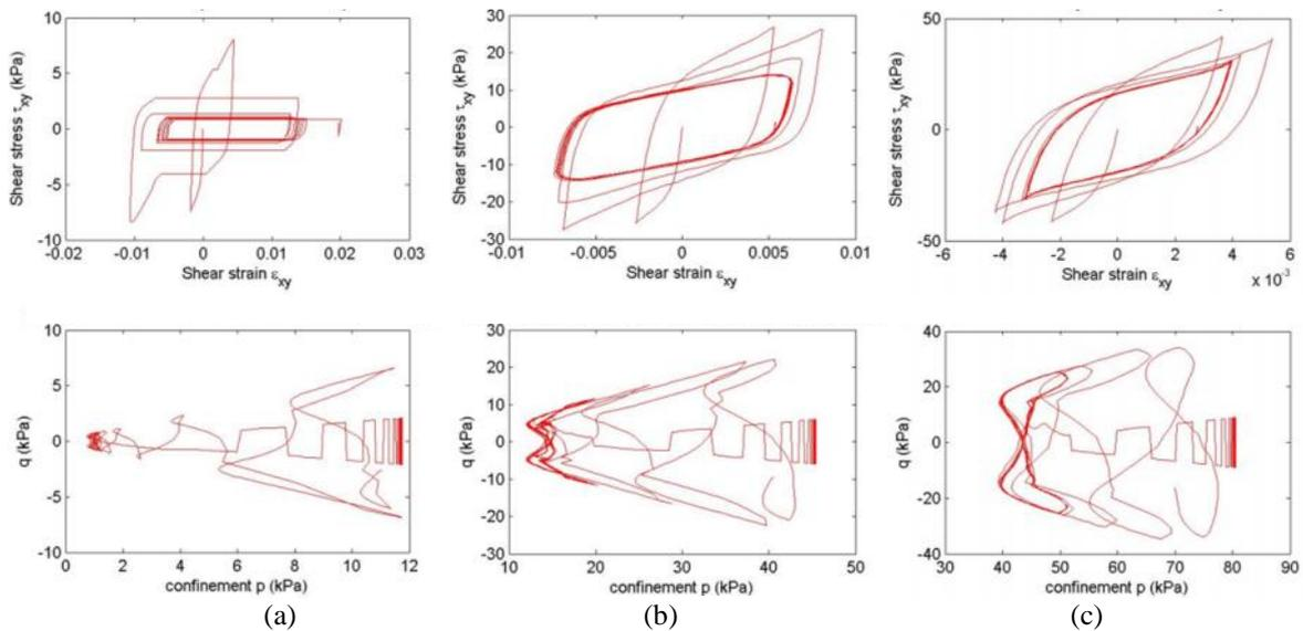
Figure 3. Shear stress  $\tau_{xy}$  VS. shear strain  $\epsilon_{xy}$  and confinement  $p$  VS. deviatoric stress  $q$  for (a) 2m depth, (b) 6m depth, (c) 10m depth, ( $k = 5e-3$  m/s, acceleration amplitude = 2, and 10 cycle)
