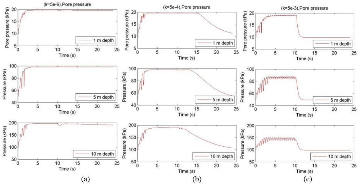
Figure 2. Excess pore pressure dissipation for (a)  $k = 5e-6$  m/s, (b)  $k = 5e-4$  m/s, (c)  $k = 5e-3$  m/s, (10 cycle, acceleration amplitude = 2)
