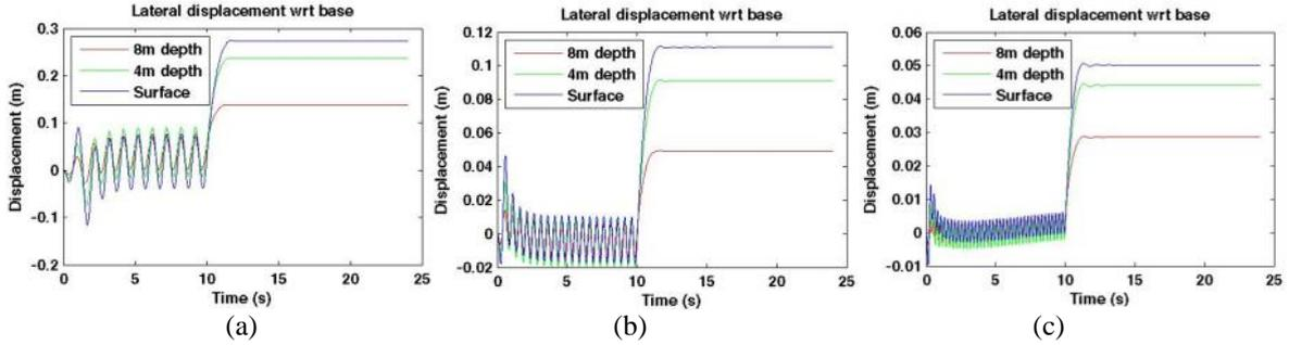
Figure 7. Lateral displacement: (a) 10 cycle, (b) 20 cycle, (c) 40 cycle, ( $k = 5e-6 \text{ m/s}$ , acceleration amplitude = 2)
