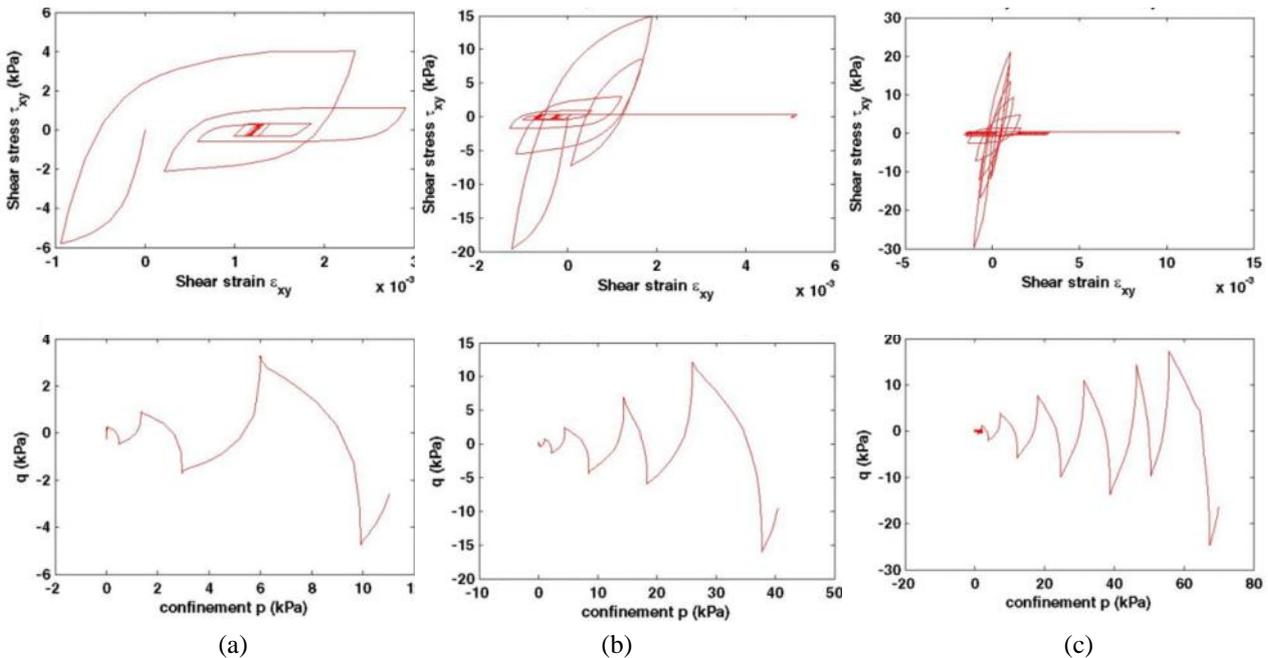
Figure 10. Shear stress  $\tau_{xy}$  VS. shear strain  $\epsilon_{xy}$  and confinement  $p$  VS. deviatoric stress  $q$  for (a) 2m depth, (b) 6m depth, (c) 10m depth, ( $k = 5e-6$  m/s, acceleration amplitude = 2, and 40 cycle)
