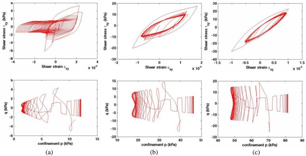
Figure 9. Shear stress  $\tau_{xy}$  VS. shear strain  $\epsilon_{xy}$  and confinement  $p$  VS. deviatoric stress  $q$  for (a) 2m depth, (b) 6m depth, (c) 10m depth, ( $k = 5e-3$  m/s, acceleration amplitude = 2, and 40 cycle)
