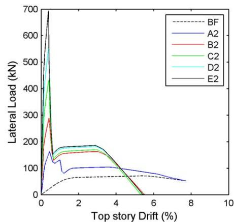
Figure 16. Push Curves (3 Story Frame, Wall Type 2)
