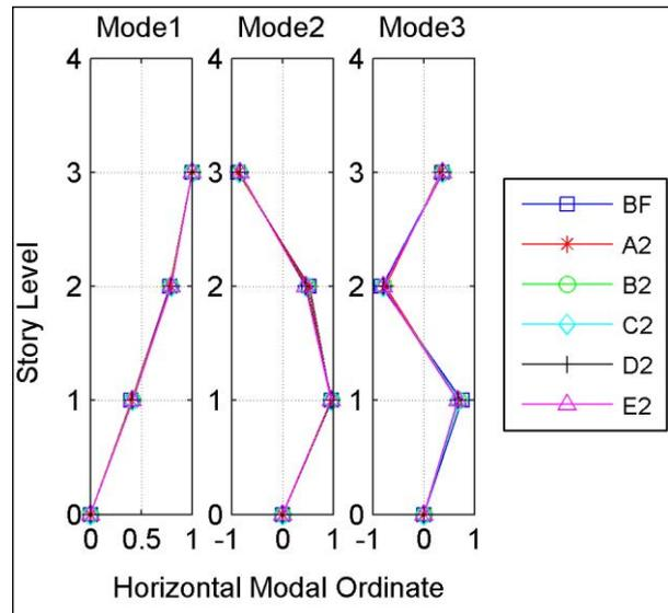
Figure 10. First Three Mode Shapes
