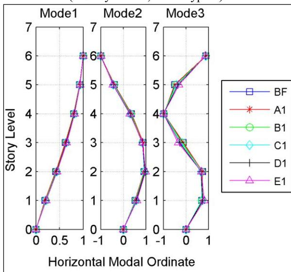
Figure 11. First Three Mode Shapes
