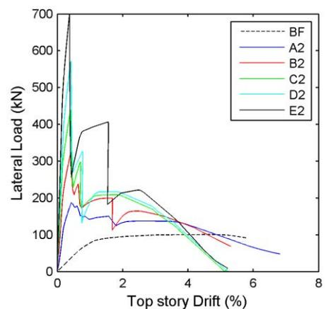
Figure 18. Push Curves (6 Story Frame, Wall Type 2)
