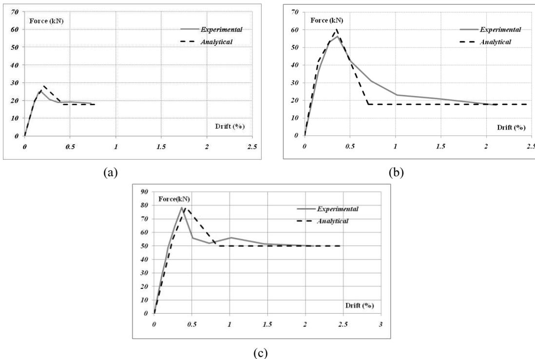
Figure 6. Comparison between experimental and analytical push curves
