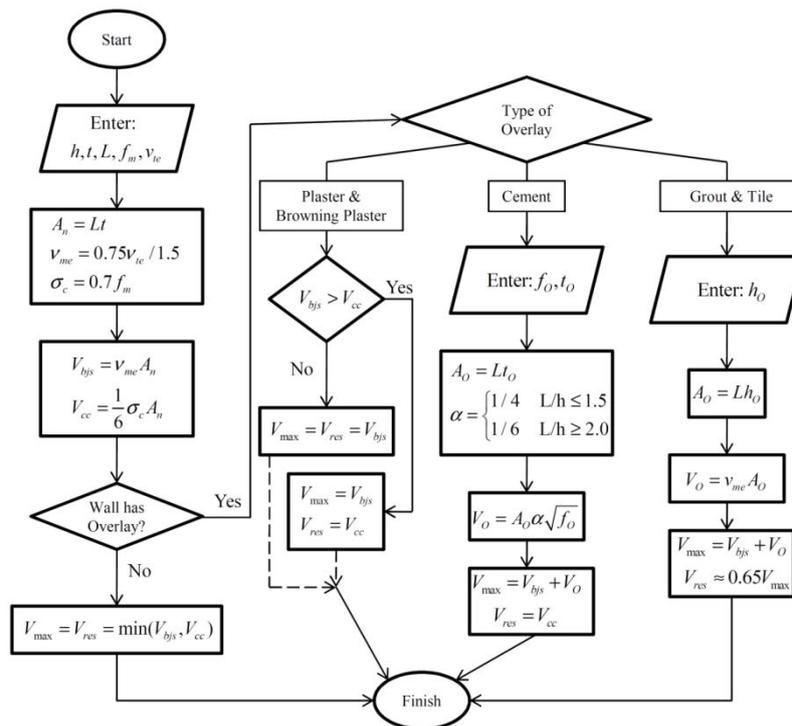
Figure 5. Maximum strength determination flowchart
