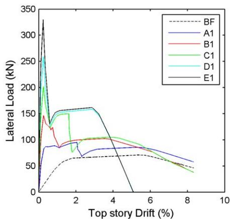
Figure 15. Push Curves (3 Story Frame, Wall Type 1)
