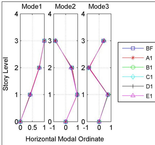
Figure 9. First Three Mode Shapes
