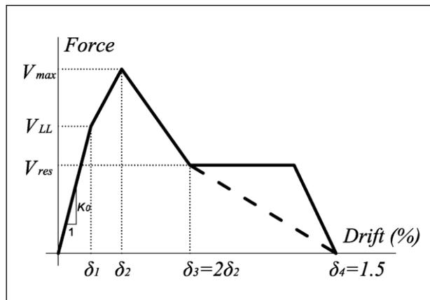
Figure 2. Typical non-linear force-deformation relation of non-structural walls developed based on experimental tests.
