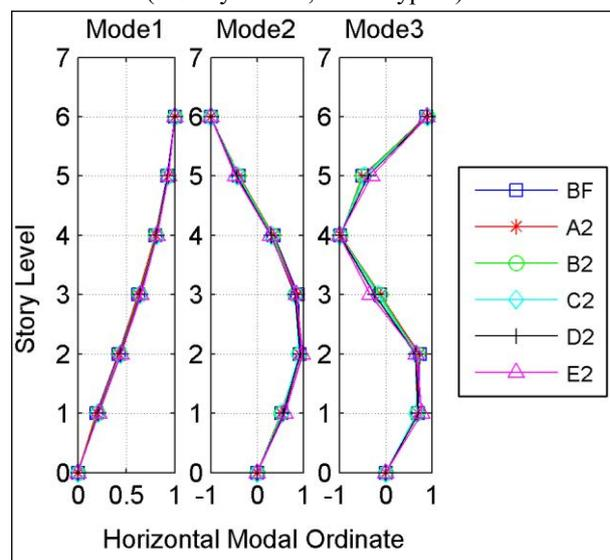
Figure 12. First Three Mode Shapes
