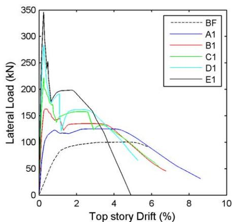
Figure 17. Push Curves (6 Story Frame, Wall Type 1)
