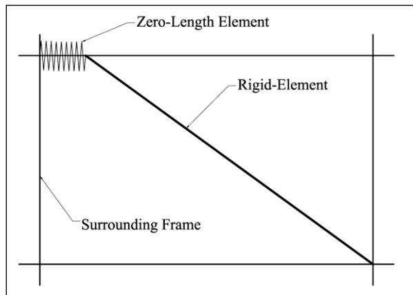
Figure 1. Rigid strut and shear spring model for wall modelling
