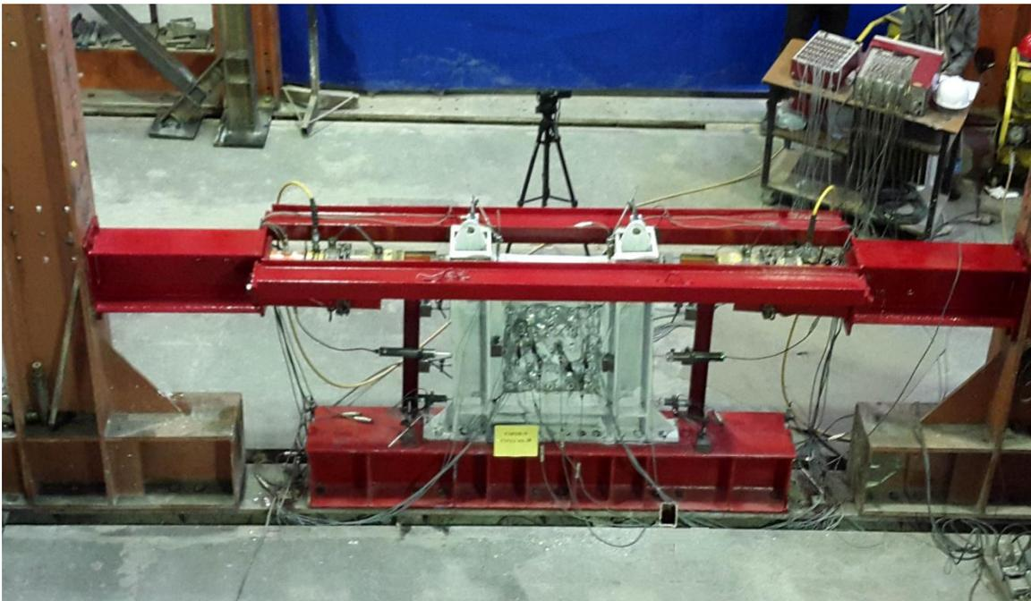
Figure 2. The dimensions of CSPSW specimen and test set up
