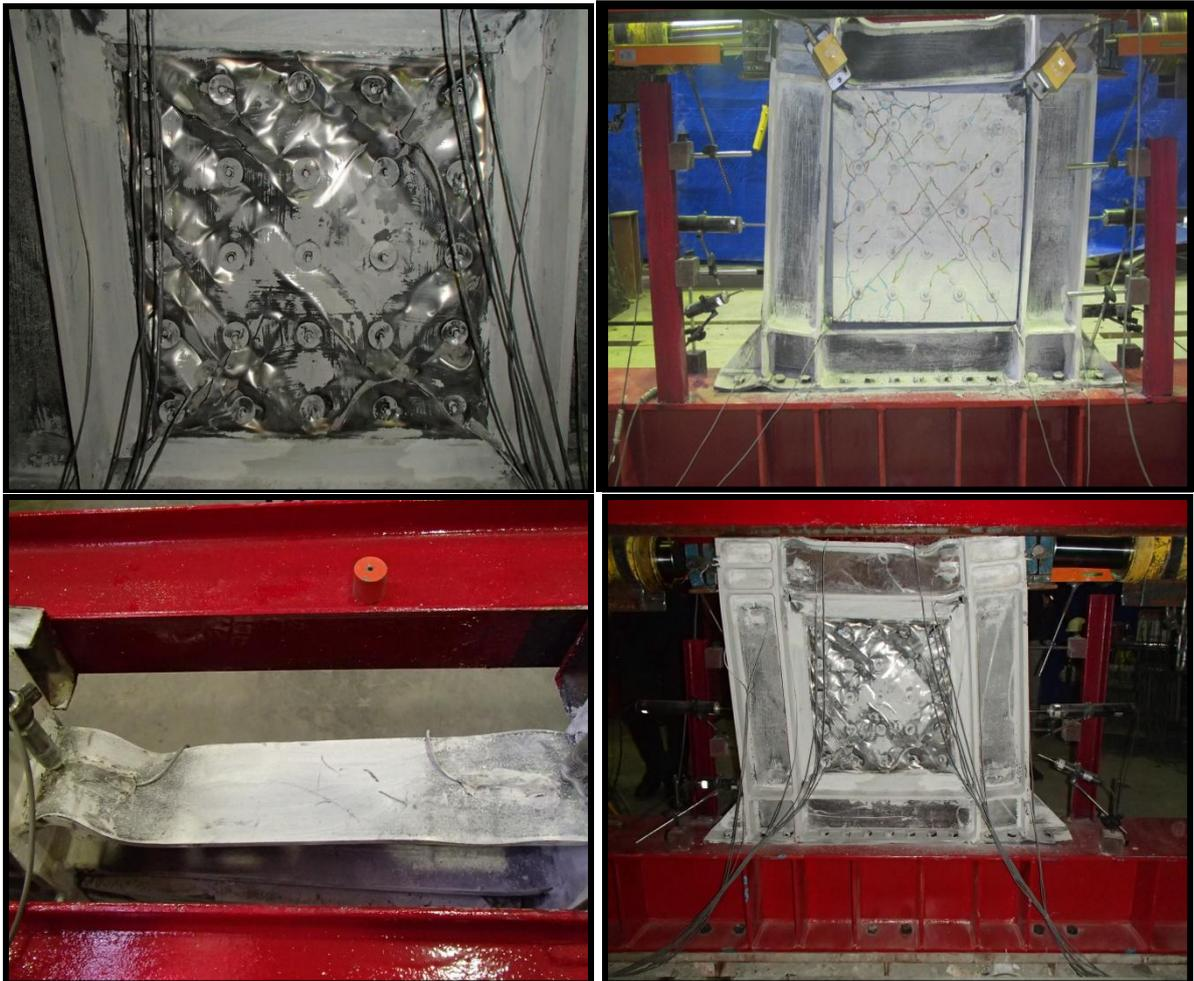
Figure 4. The CSPSW specimen after the test
