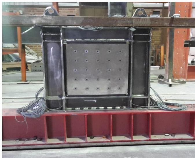
Figure 1. The one-story one-bay CSPSW specimen
