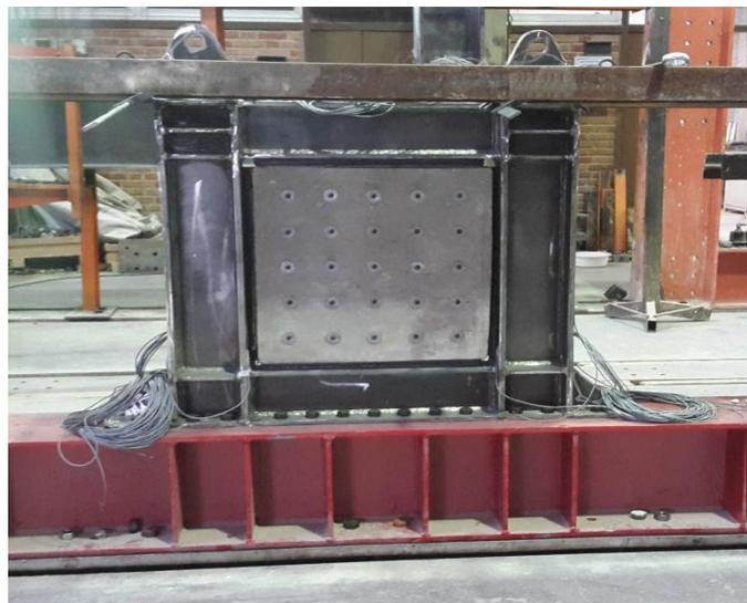
Figure 1. The one-story one-bay CSPSW specimen
