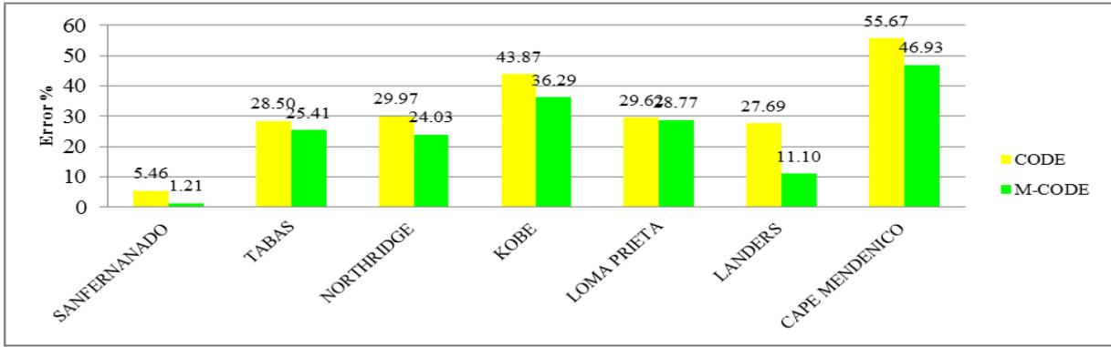
Figure 4. Code and M-Code Maximum error in beam plastic hinge rotation for SAC9 subjected to seven near-field ground motions
