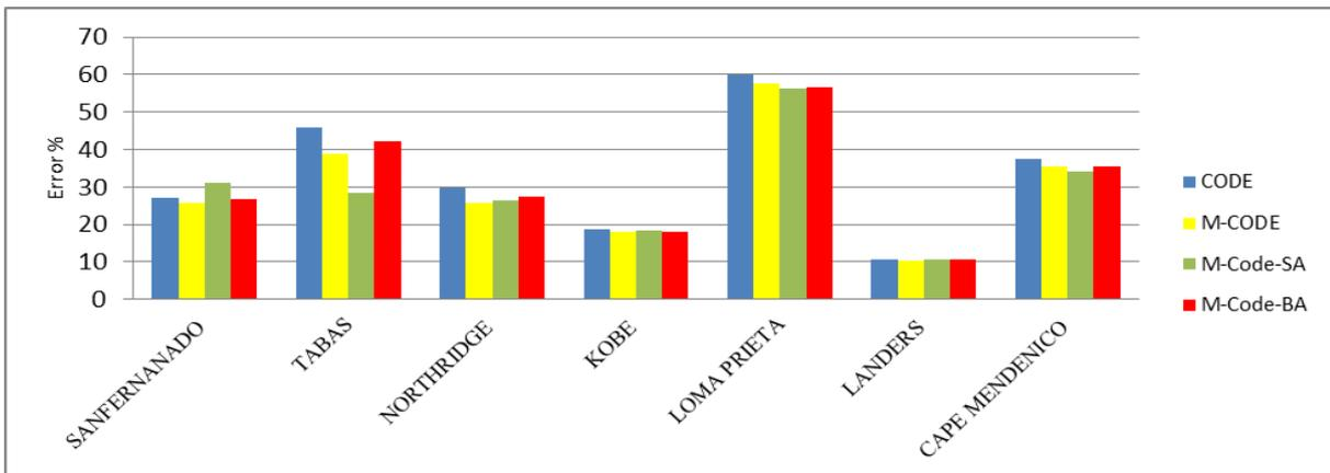
Figure 6. Overall Comparison of Code, M-Code, M-Code-SA and M-Code-BA Maximum error in beam plastic hinge rotation for SAC9 subjected to seven near-field ground motions
