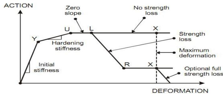
Figure 1. Nonlinear behaviour curvature (PERFORM 3D, 2006)
