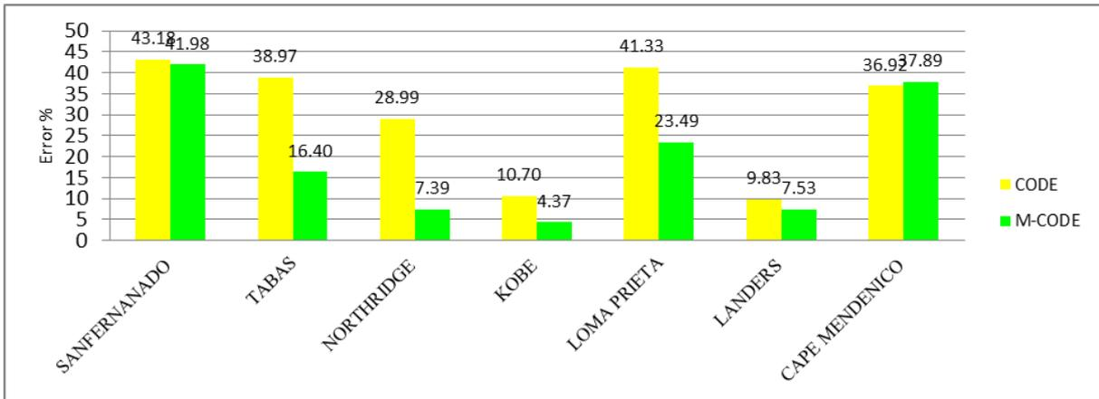
Figure 5. Code and M-Code Maximum error in column plastic hinge rotation for SAC9 subjected to seven near-field ground motions
