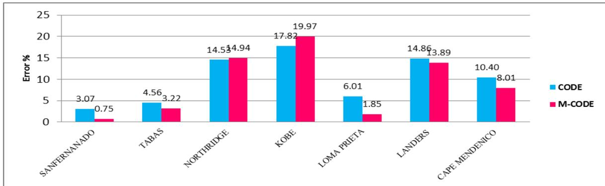
Figure 2. Code and M-Code Maximum error in beam plastic hinge rotation for SAC3 subjected to seven near-field ground motions
