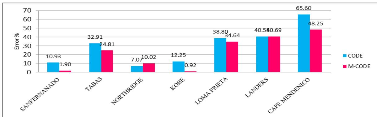
Figure 3. Code and M-Code Maximum error in column plastic hinge rotation for SAC3 subjected to seven near-field ground motions
