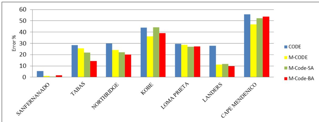
Figure 7. Overall Comparison of Code, M-Code, M-Code-SA and M-Code-BA Maximum error in column plastic hinge rotation for SAC9 subjected to seven near-field ground motions
