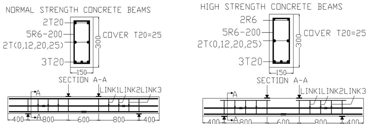
Figure 2: Geometry, Reinforcement details and position of strain gauges for all the Normal and High Strength Concrete for all test specimens other than NSCL and BJ-2 which have similar geometry for beams but their detailing is shown in Table 1. Horizontal Web Bars (HWB) are located at half the depth and are 2T (12,20 & 25).
