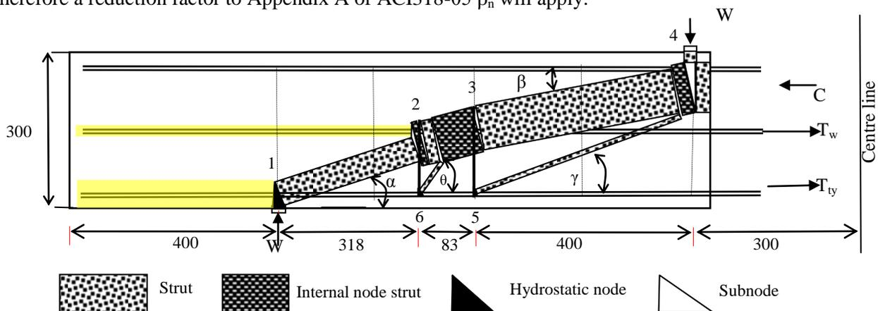
Figure 4: Strut-and-tie model for HSC beam with HWB of  $a/d=3.02$  with stirrup. The sum of the shear transmitted is counter balanced by vertical components of the deflected strut which has an improved arching action as well as by the stirrups.
