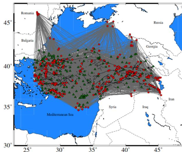
Figure 1. Ray coverage for  $M_L$  amplitude readings. The grey lines are the surface trace of the event-station paths; red circles are epicenters of the selected events, green triangles are seismic stations, the black lines are simplified traces of active faults and the dashed grey lines are political borders.
