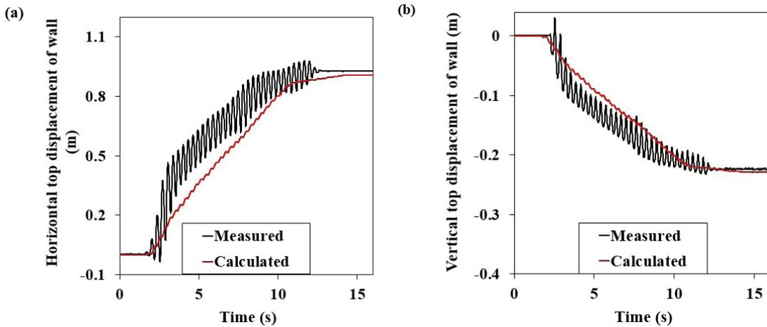
Figure 3. Deformation time histories: (a) horizontal and (b) vertical displacements at top of quay wall.
