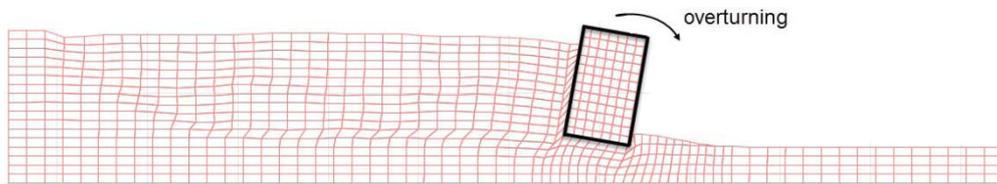
Figure 4. Deformed configuration of wall–soil system at the end of shaking.
