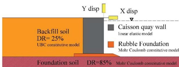
Figure 1. Schematic cross section of quay wall.
