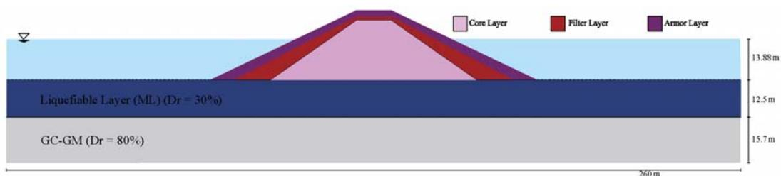
Figure 1. Schematic of breakwater and foundation soil layers and input acceleration wave.
