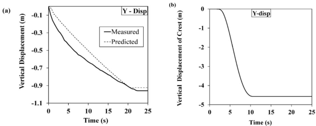
Figure 3. (a) Comparisons between the computed and measured results; (b) vertical displacements of breakwater crest after seismic loading.
