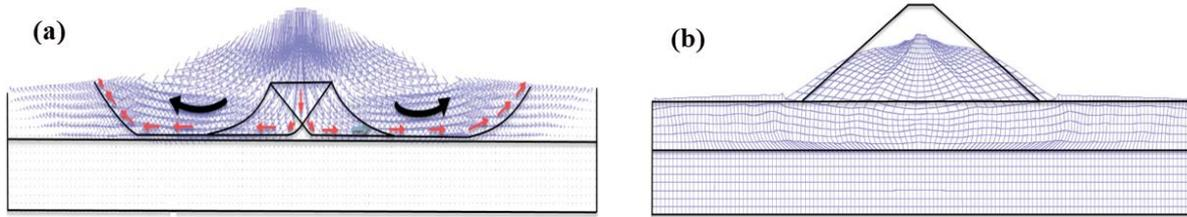
Figure 2. Results of seismic response: (a) displacement vectors, and (b) deformed configuration of rubble mound breakwater after earthquake loading.
