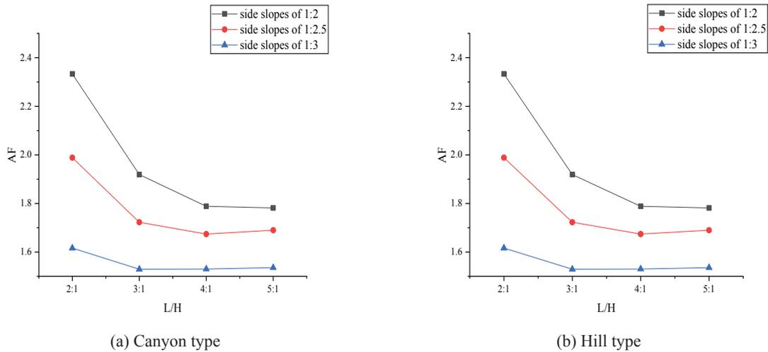
Figure 2. Amplification factor results for Canyon and Hill types in various  $V/H$  and  $L/h$  ratios.
