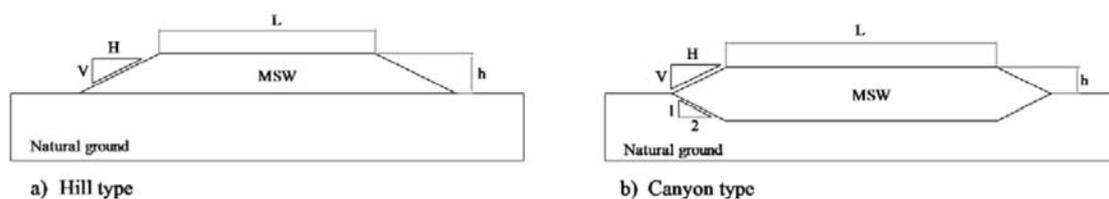
*Figure 1. Typical MSW landfill geometries used in the numerical analysis: a) Canyon type, b) Hill type.*
