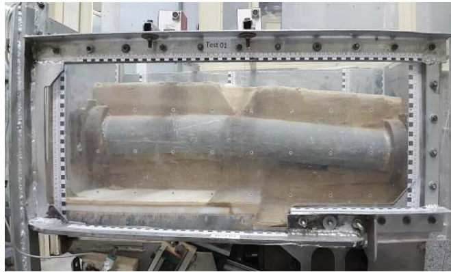
Figure 2. Longitudinal view of damaged tunnel subjected to reverse faulting.
