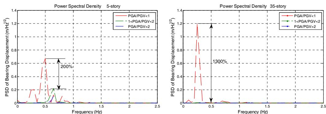
Figure 2. Power spectral density of bearing displacement for both low-rise and high-rise base-isolated buildings.
