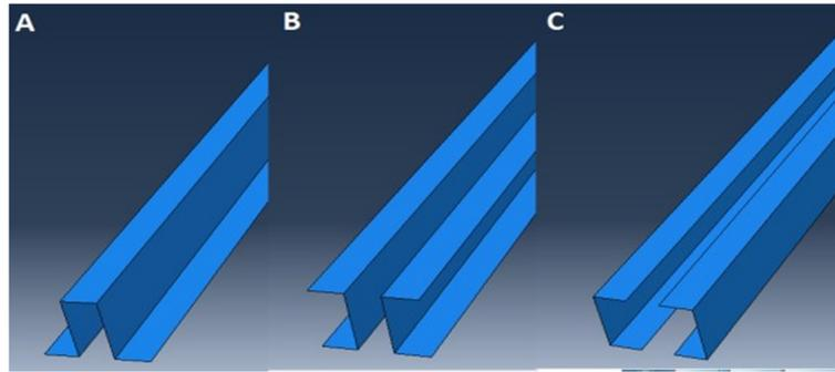
Figure 1. Different geometries used for the buckling restrained core.
