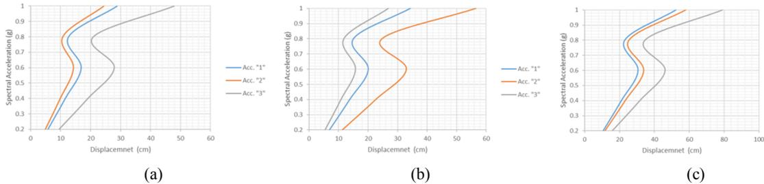
Figure 3. Diagrams of Spectral Acceleration versus Displacement for Filling Strategy of 100% for soil categories of: a) Rock, b) Dense Soil and c) Loose Soil for model "a".
