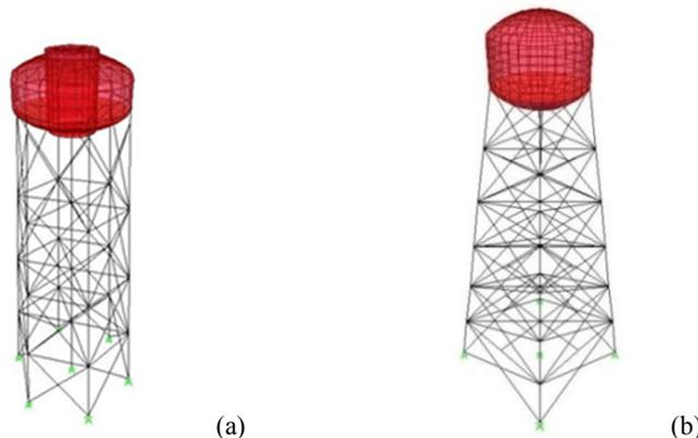
Figure 1. Numerical Models: (a) 134 m<sup>3</sup> & h=24.0 m, (b) 160 m<sup>3</sup> & h=30.0 m.
