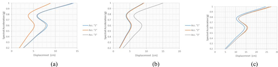
Figure 4. Diagrams of Spectral Acceleration versus Displacement for Filling Strategy of 50% for soil categories of: a) Rock, b) Dense Soil, and c) Loose Soil for model "b".
