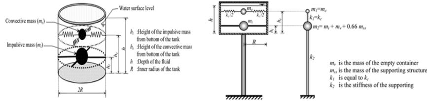
Figure 2. Two mass model and equivalent Mass-Spring.
