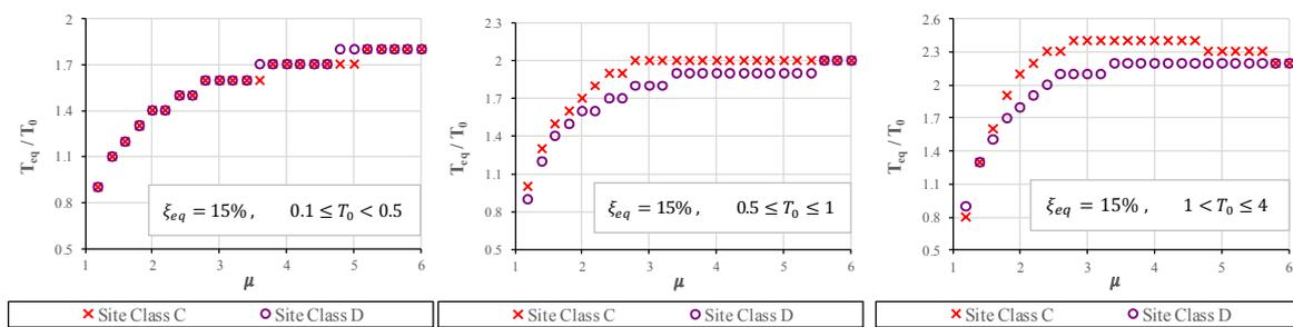
Figure 1. Soil type effects on equivalent period ratio of BLH models for equivalent damping of 15%.
