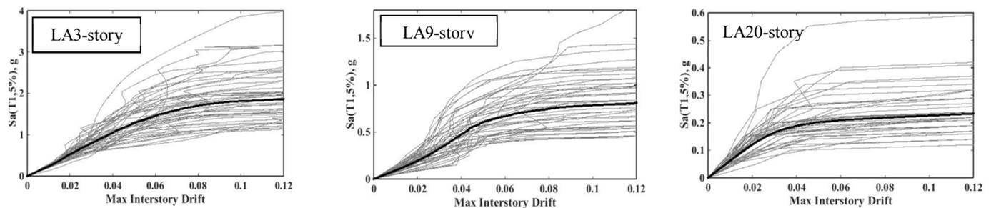
Figure 3. IDA and median curves of SAC buildings with bilinear with deterioration behavior.
