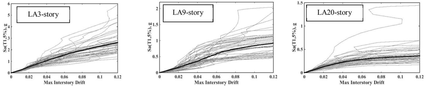
Figure 2. IDA and median curves of SAC buildings with elasto-plastic behavior.
