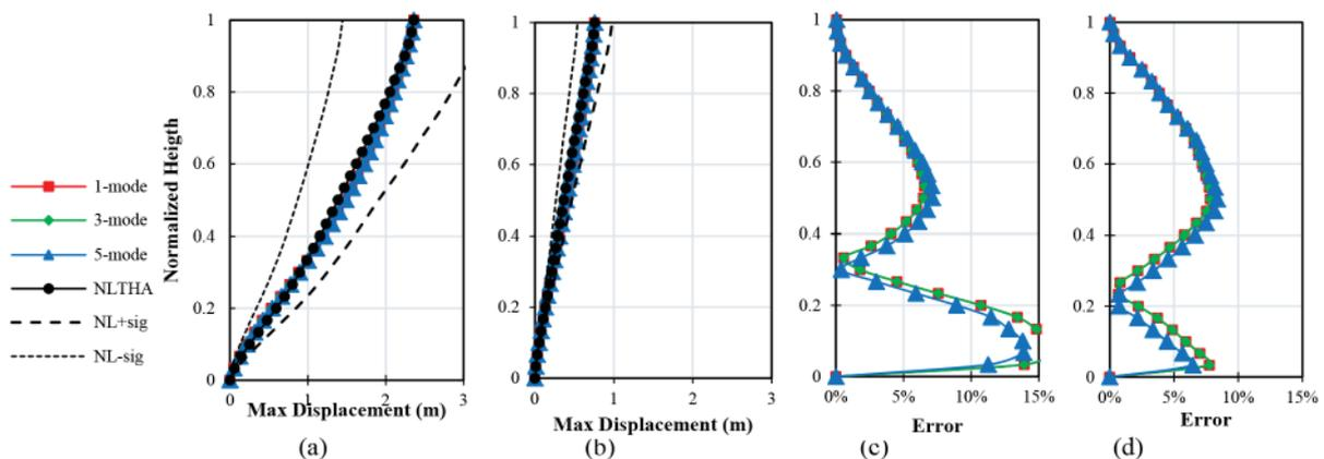
Figure 2. The mean values of the maximum lateral displacement related to floor mass centre (CM) of the CT model in y direction of plan (Figure 1); (a) the near field records, (b) the far field records, and the relative error due to the estimated response parameter under; (c) the near field records, (d) the far field records.
