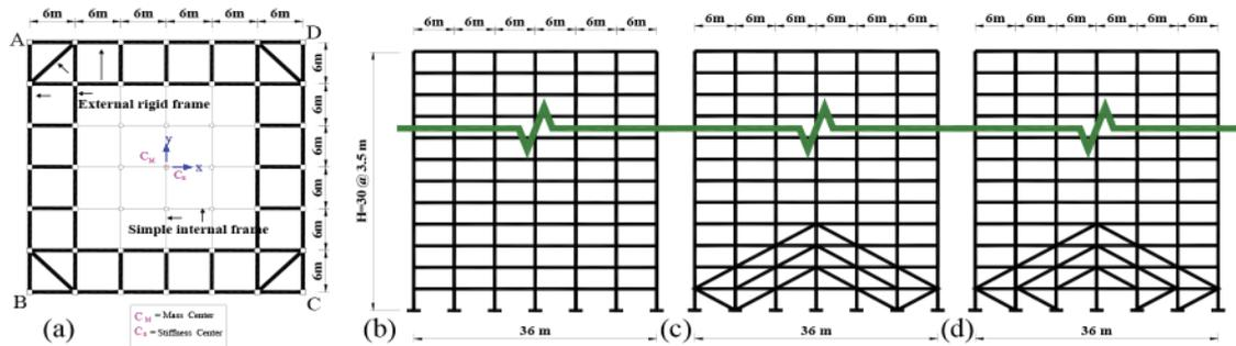
Figure 1. The structural configuration of the studied models: (a) The plan of castled tube skeleton; (b) The CT model; (c) The MZCT-2C model; (d) The MZCT-1C model.
