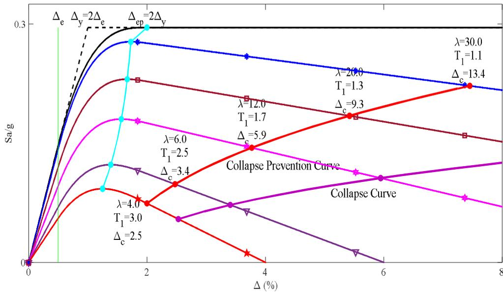
Figure 1. Pushover results for a typical 4 story frame structures.
