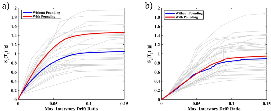
Figure 1. IDA curves of the 4-Story RC SMRF, section a, pounding with the 9-Story steel SMRF, section b, with clear distance of 1.0D subjected to 28 near-field earthquakes having pulse subset.
