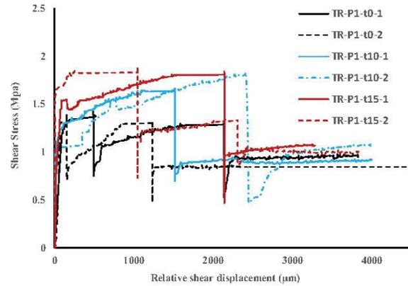
(b) Shear stress versus shear deformation
