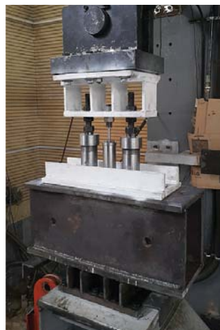
Figure 1. Test setup for the self-centering energy dissipater.
