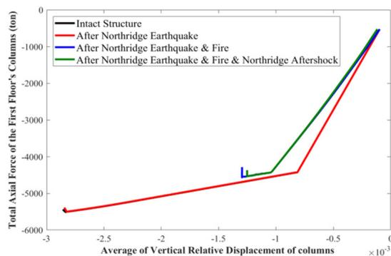
Figure 2. Total axial force versus average of downward relative displacement in the first floor's columns in the pushdown analysis after each step.
