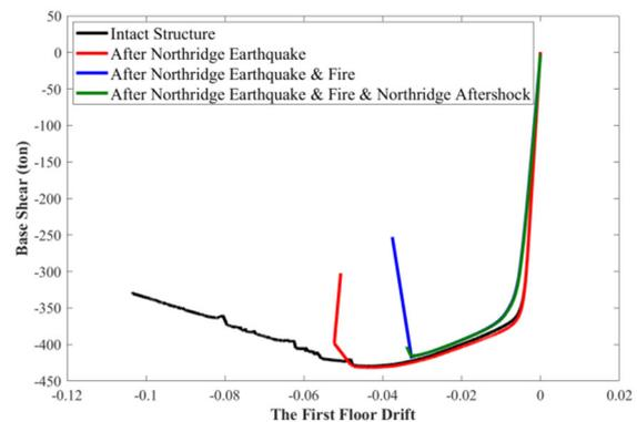
Figure 3. Base shear versus the first story drift in the pushover analysis after each step.
