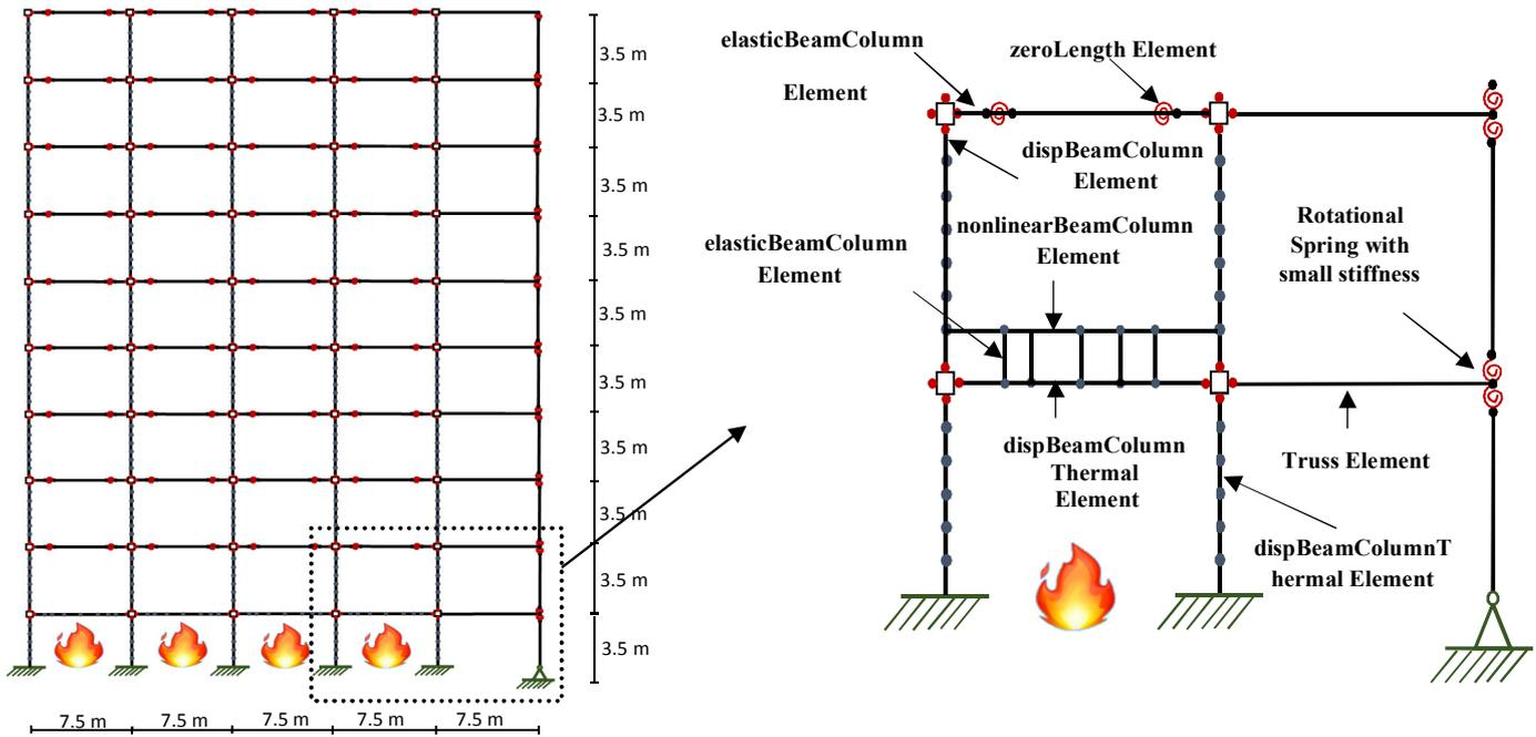
Figure 1. (Left): Case study building geometry, (Right): Analytical model in OpenSees.
